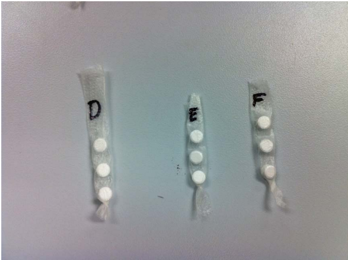
Figure 3 Pellet dosimeters in wrapping for internal dose measurement
