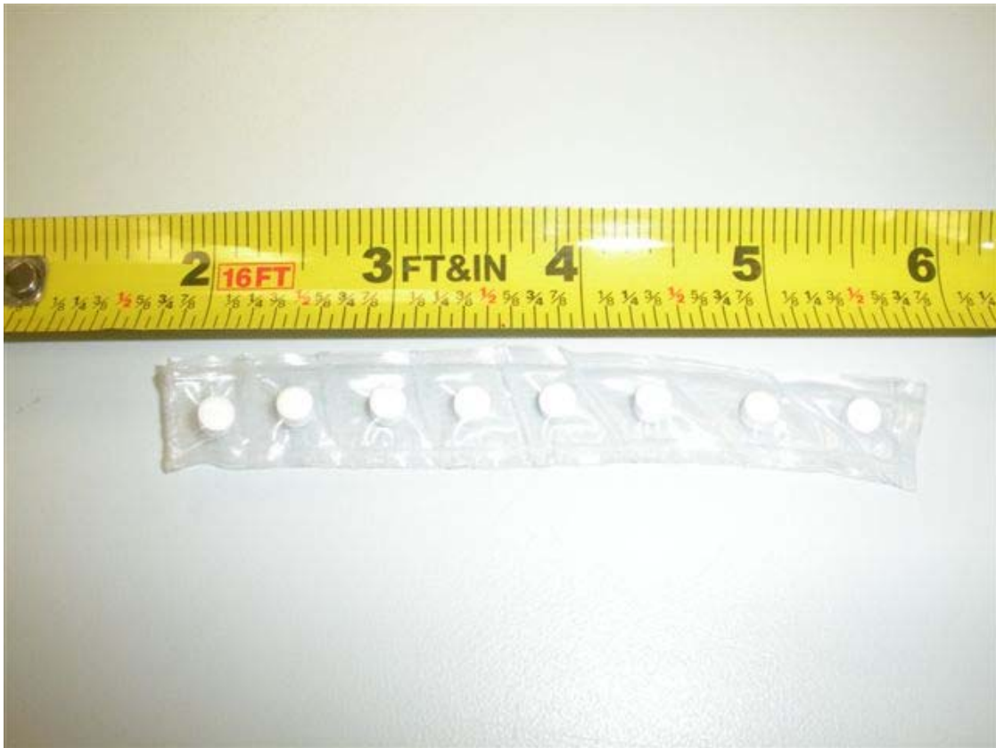
Figure 4 Pellet dosimeters bagged for internal dose measurement
