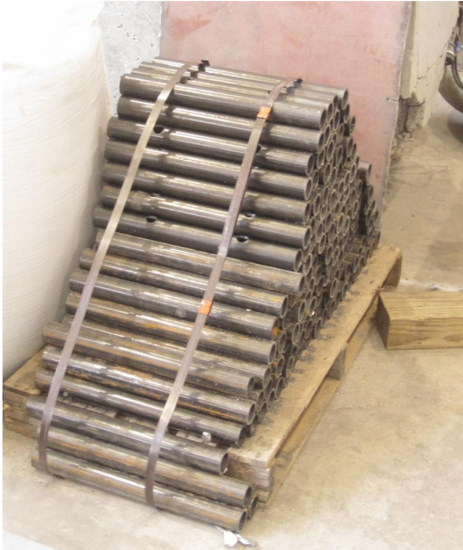
Figure 12 Steel pipes used for anchorage
