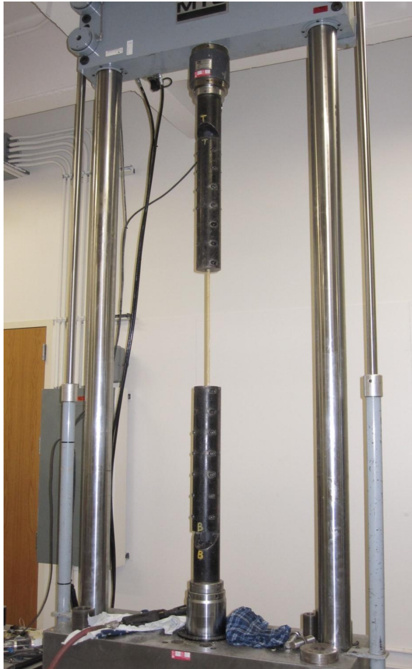
Figure 22 Grouted steel pipe anchorage system tensile test
