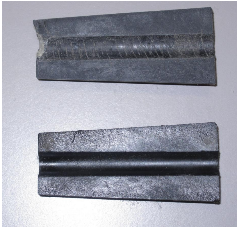
Figure 10 Plastic wedge roughened surface and regular surface
