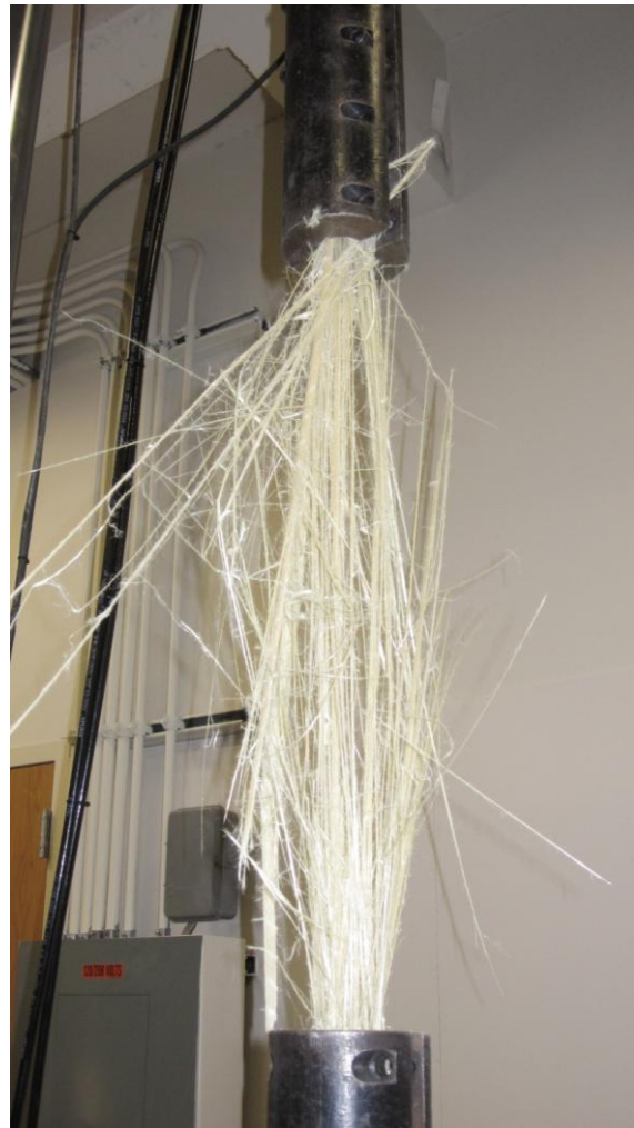
Figure 24 Tensile failure of AFRP bar using grouted steel pipe anchorage system
