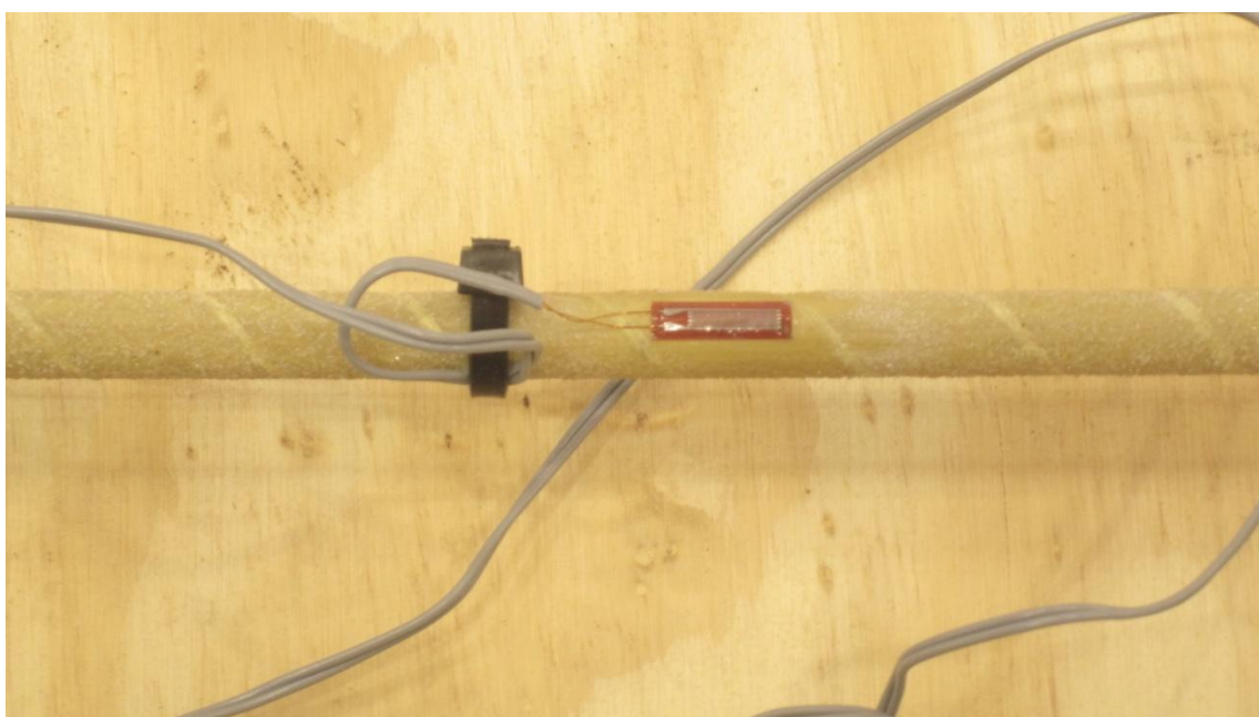
Figure 16 Strain gauged AFRP bar
