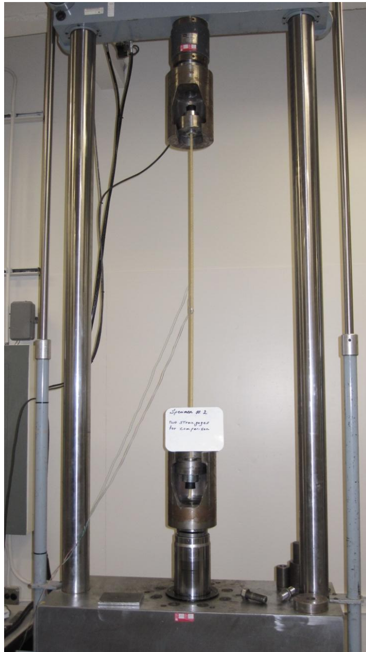
Figure 9 Conventional anchorage system tensile test setup
