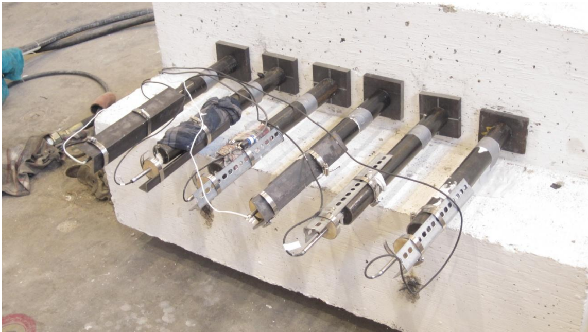
Figure 76 Live ends with LVDTs
