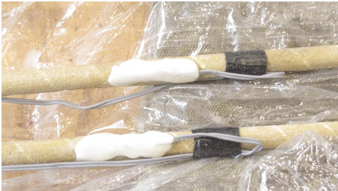
Figure 73 Concrete protected coating on strain gauges
