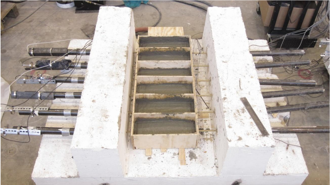
Figure 75 Long-term relaxation bars with concrete
