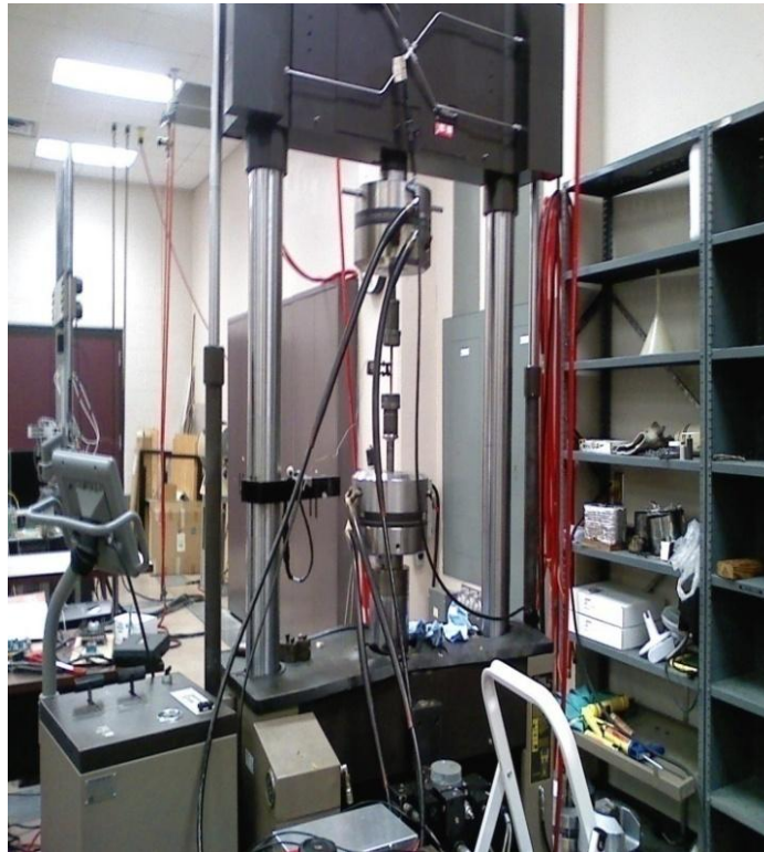
Figure 29 Tensile testing machine and rod specimen setup
