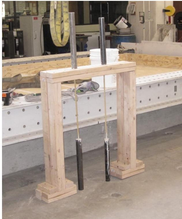
Figure 21 Wooden frame holding grouted AFRP specimens
