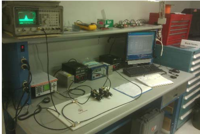
Fig. 14 Packet Loss Rate (PLR) testing arrangement implementation.
