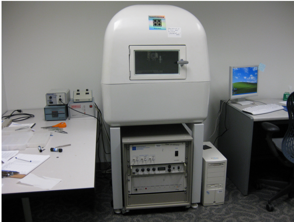
Figure 13: The nanoindenter used in this study was the Hysitron Triboindenter. This device is a flexible, stand-alone nanomechanical testing system and is widely considered the industry standard for nanoindentation testing.
