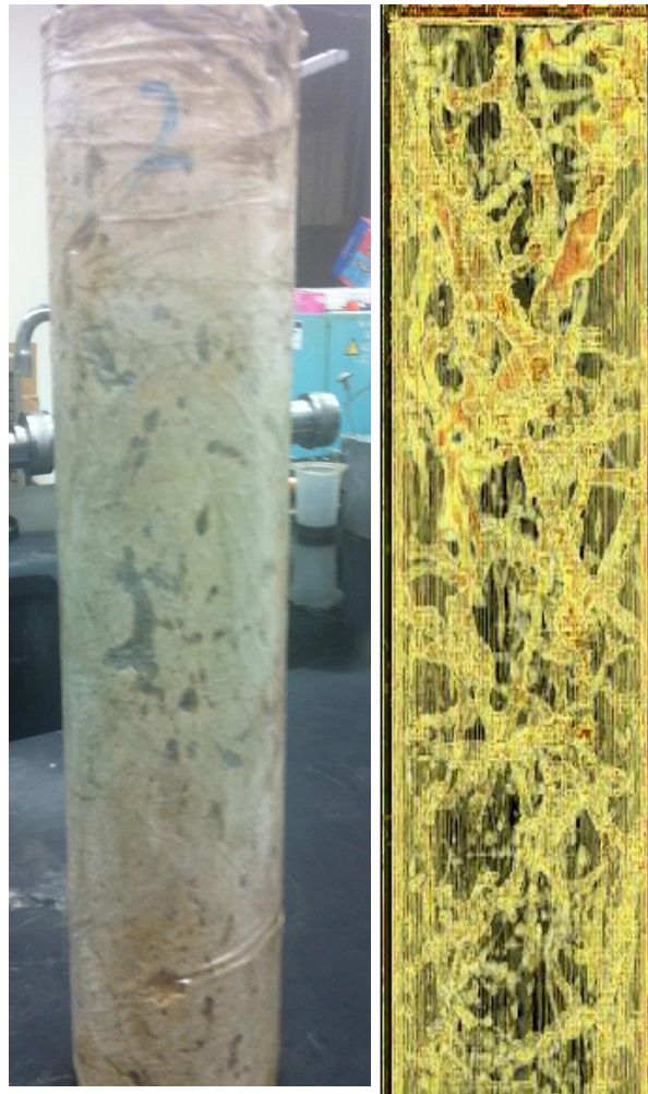
Fig. 3.15—Core with Drill-in Fluid Contamination
