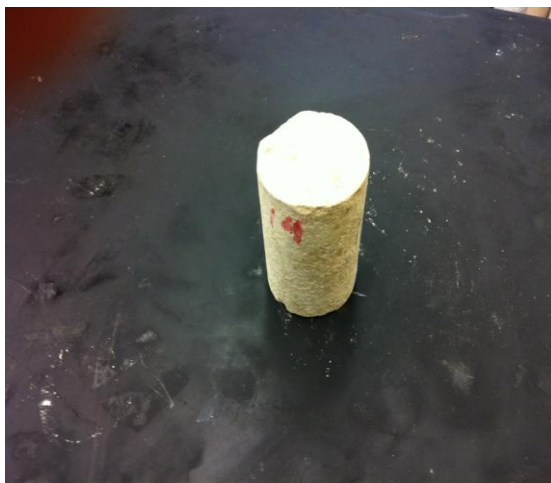
Fig. 2.6—Homogenous Core before Acidizing Experiment
