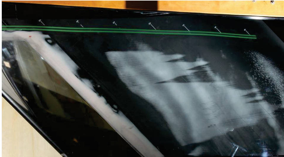
Figure 5-17. Naphthalene flow visualization of natural transition at TAMU for Re_c = 2.8 \times 10^6 , \alpha = -2.9^\circ ; wall-liners installed.
