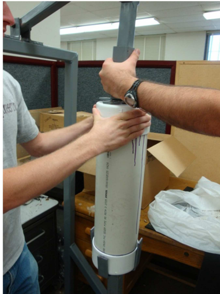
Figure 4. Cotton being sealed in plastic tube for storage.
