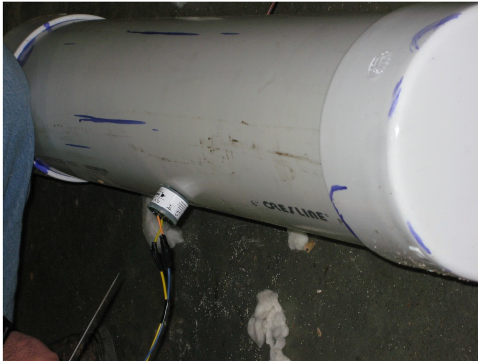
Figure 13. Oxygen sensor is installed on a seed cotton sample.
