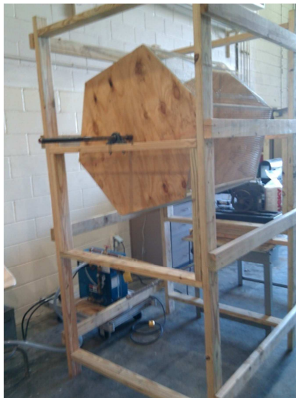
Figure 14. Moisture addition system for Test 2. Moisture was added during the second series of tests using a large basket with the outlets of the steam generator placed directly beneath it. This container was wrapped in plastic (removed for picture) so that the steam exited through the seed cotton samples and the top of the frame.
