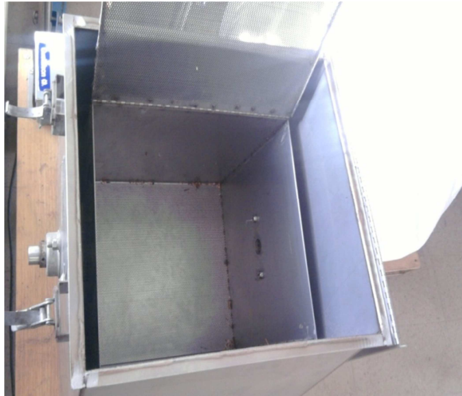
Figure 2. Air wash system used to increase moisture contents of test samples. The basket containing the samples was rotated while steam was pulled through the pipe axle (not shown) and the cotton samples.
