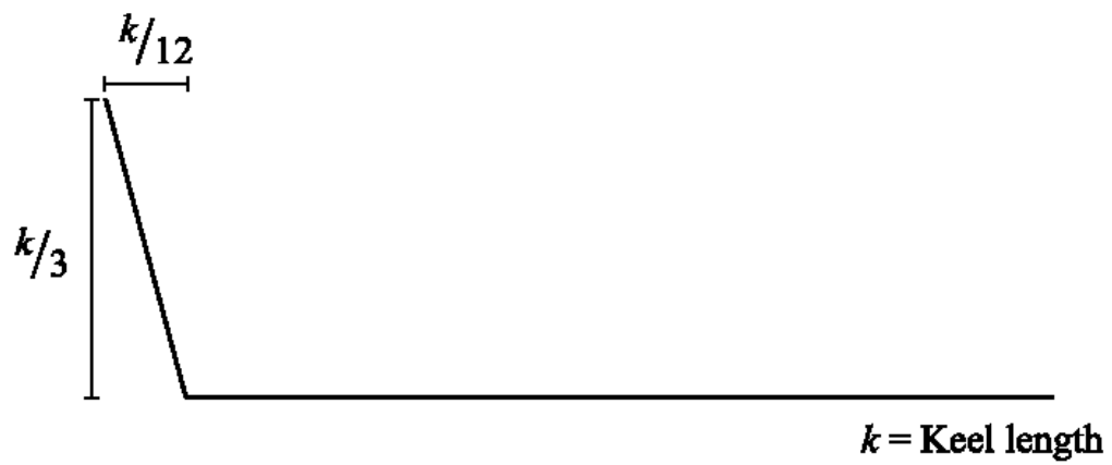
Figure 8. Drawing of sternpost based on Oliveira. This image shows the keel and the sternpost.
