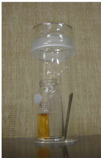
Fig. 48. Capillary condensation setup. Substance to be condensed (colored orange for clarity) in a 2\text{ mL} glass vial is placed inside a secondary 20\text{ mL} glass vial, and then inside a large weighing bottle containing the substrate.
