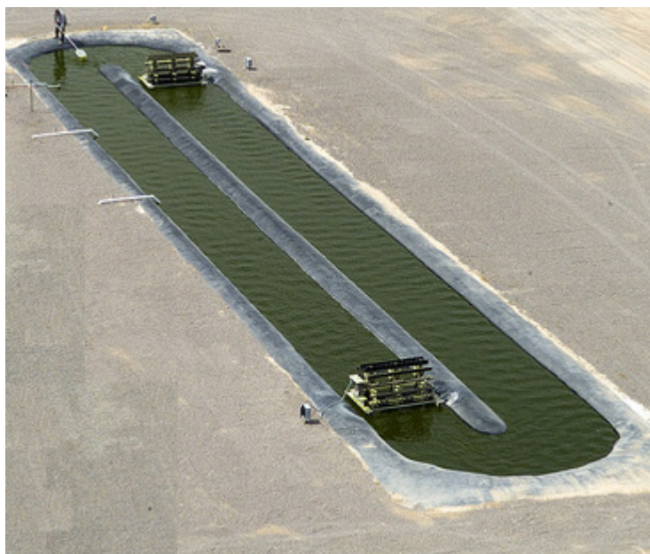
Figure 7. Depiction of a raceway photo-bioreactor. Source: AGLR, 2011
