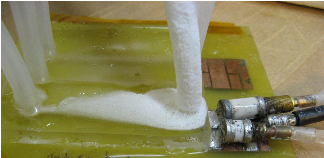
Fig. 11 35 \mu\text{m} copper etched planar pair coil with PDMS microfluidic channel attached. The coil is being cryo-cooled by gravity-fed liquid nitrogen through the PDMS channel. Ice formation is evident on the liquid nitrogen inlet.
