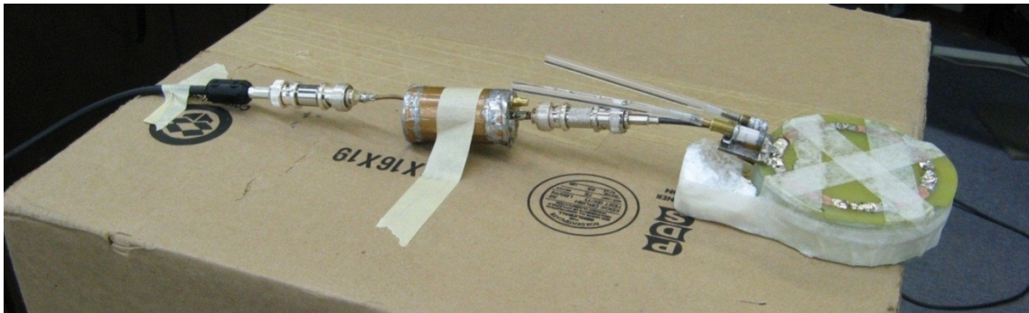
Fig. 4 Coil, matching network, and balun test setup for S_{11} 7 dB return loss measurement.
