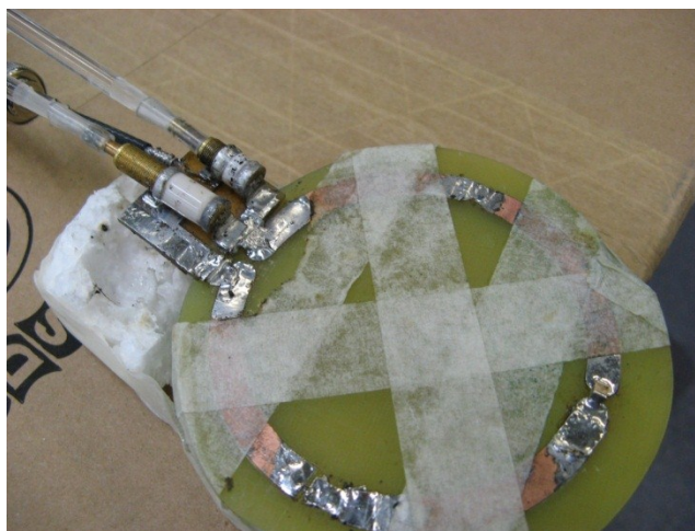
Fig. 3 Coil (8 cm diameter) and matching network used for validation of 7 dB return loss Q measurement.
