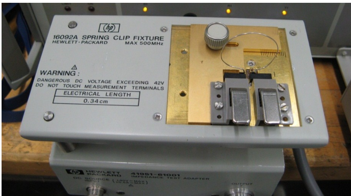
Fig. 17 HP 41951A impedance test kit. This photograph shows a 1 inch diameter single turn coil placed in the fixture instead of a varactor diode.
