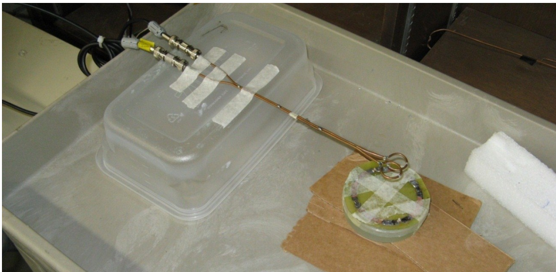
Fig. 5 Coil resonated with fixed capacitors, with the matching network removed. Dual probes are used to measure Q with an S_{21} transmission-type measurement.
