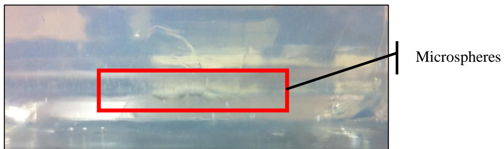
Fig. 38. Cross section image of the non-agar phantom, showing placement of microspheres.
