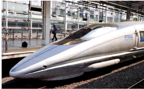
Figure 6: The shape of the Shinkansen train's nose is inspired by the Kingfisher's beak
