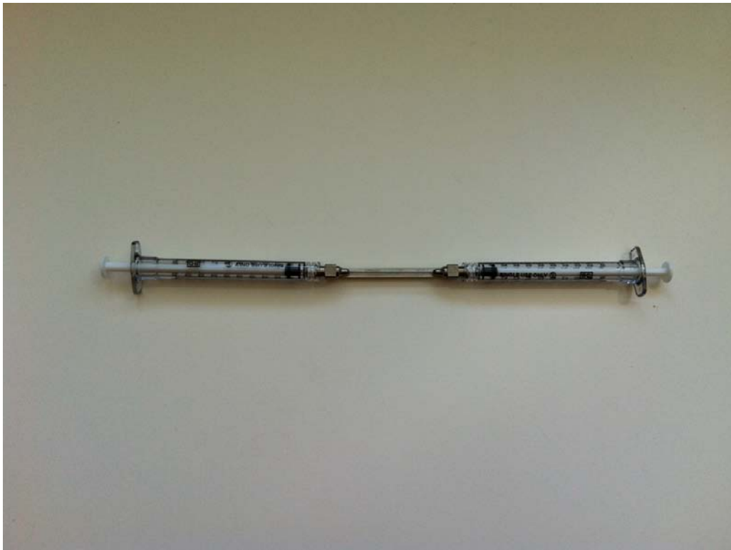
Figure 3: Emulsifying Needle. Demonstration of Emulsifying Needle with Two 1.0 ml Luer-lock Syringes for Intraperitoneal Antigen Delivery.
