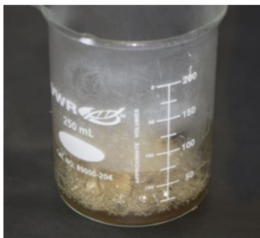
Fig. 15 —Spending formic acid in a beaker by adding pieces of carbonate rock.
