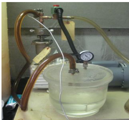
Fig. 5—Core saturation vacuum pump setup
