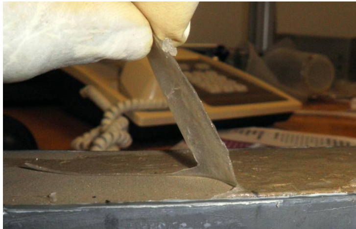
Fig. 1—Filter cake on core face
