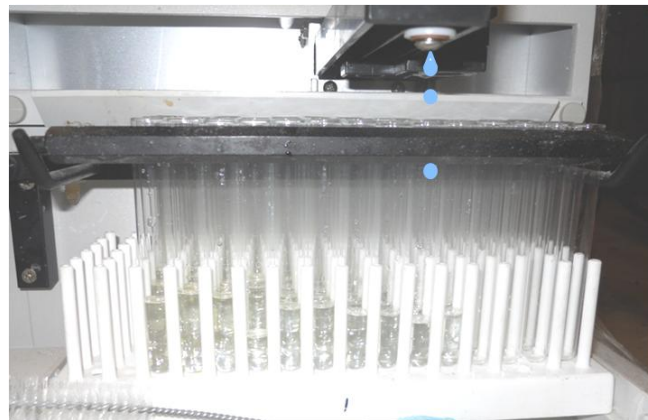
Fig. 15—Fractional collector showing clear leak off fluid (water)
