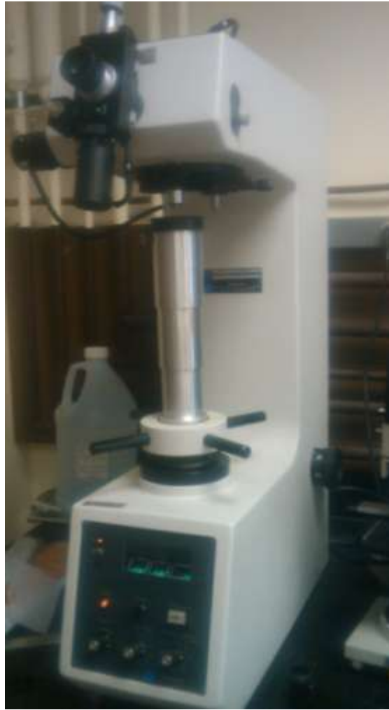
Figure 6. Experimental set-up for Vickers hardness tester
