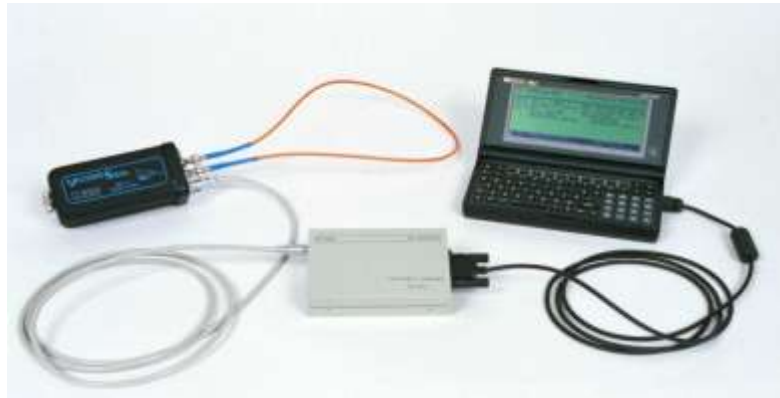
Figure 1. A VACOSS system shown connected to a laptop 3
