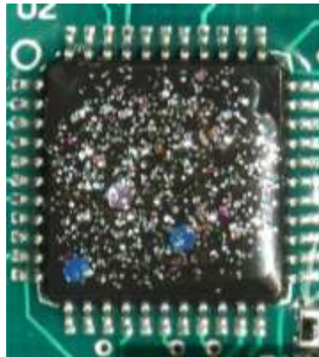
Figure 3. A reflective particle tag applied to a circuit board component 5
