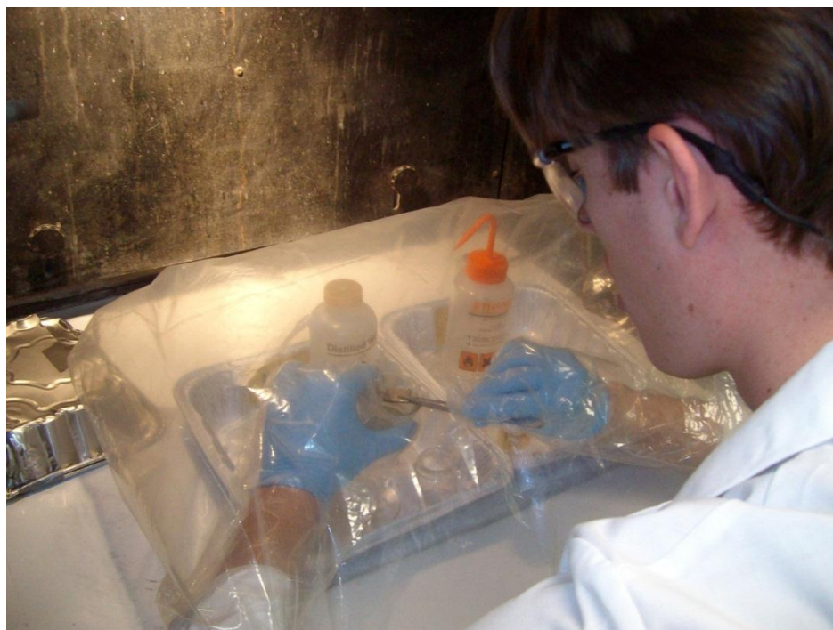
Figure 11. Acid wash station located inside a glovebag under argon atmosphere to reduce sample oxidation.
