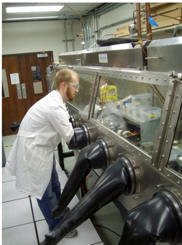
Figure 14. Glovebox in operation, working at the hydride-dehydride station.
