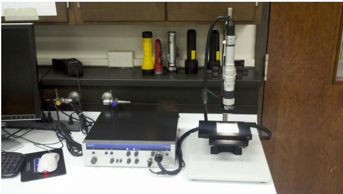
Figure 7. HIROX digital microscope used for powder imaging.
