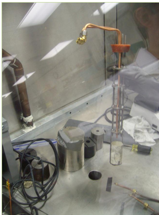
Figure 12. Aluminum oxide crucible located at the bottom of the hydride-dehydride rig.
