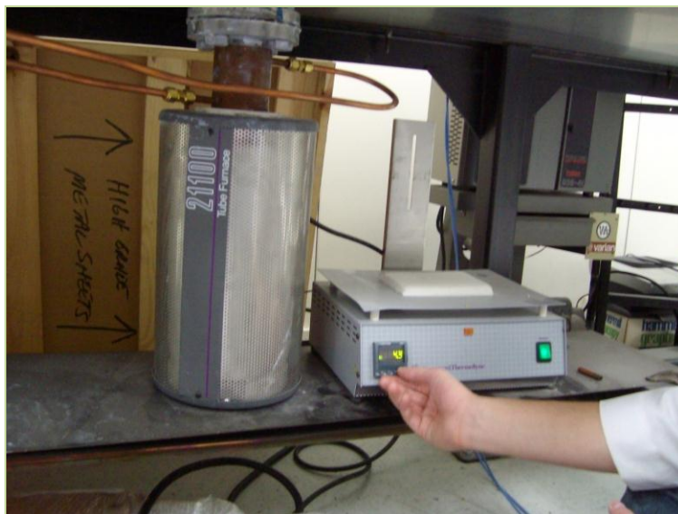
Figure 13. Furnace and furnace controls used in hydride-dehydride process.
