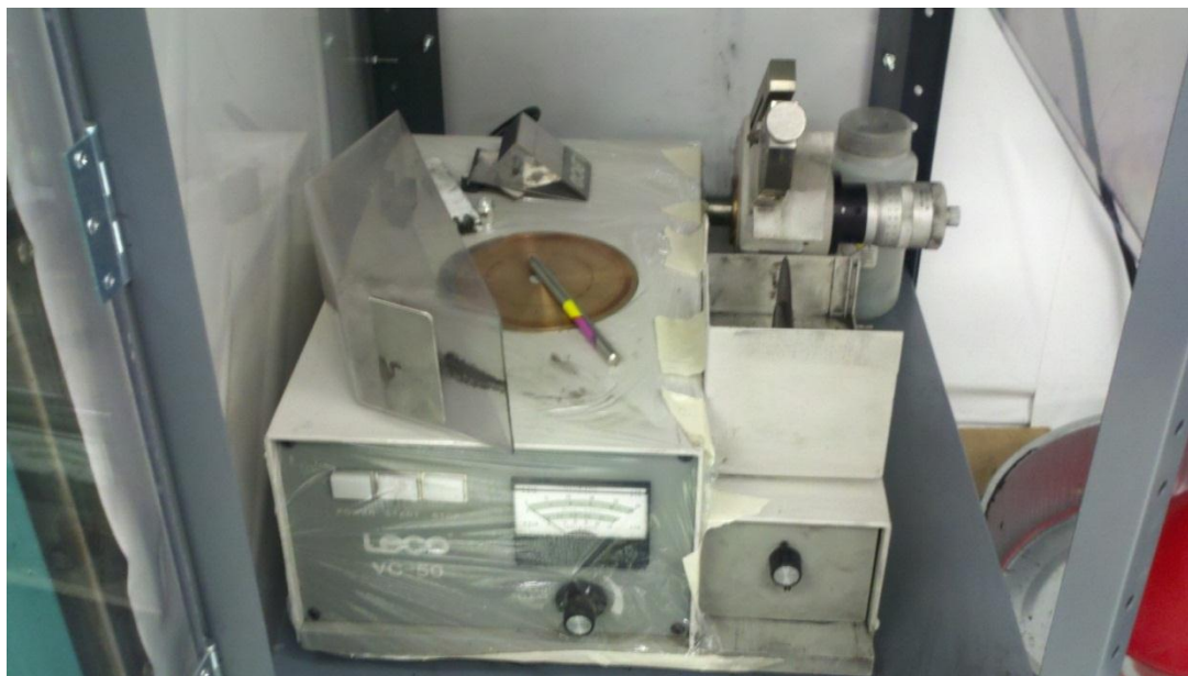
Figure 9. Diamond saw used for cutting uranium metal slugs into smaller sample sizes.
