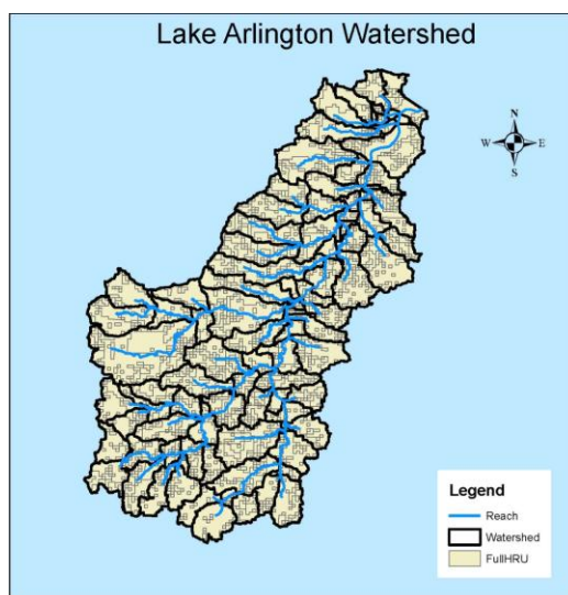
Figure 1. Hydrological model of the drainage area flowing into Lake Arlington.
