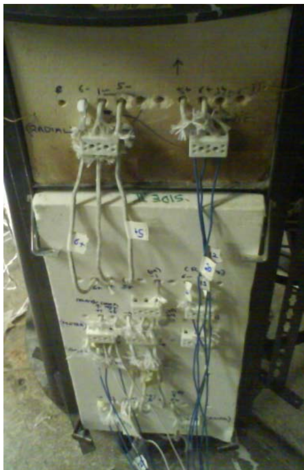
Figure 4-38 High temperature terminal blocks mounted on Zircar insulation pads
