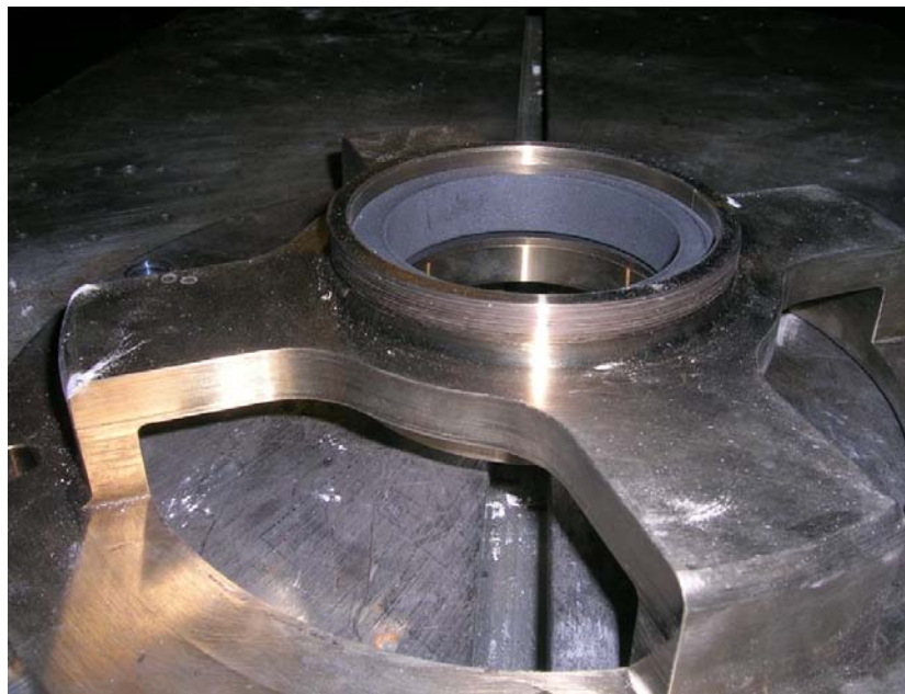
Figure 4-8 Graphalloy shrink-fitted within the catcher bearing stator plate
