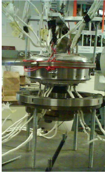
Figure 4-12 Bottom radial bearing being guided on the corresponding stator plate (with the bottom catcher bearing stator plate attached).
