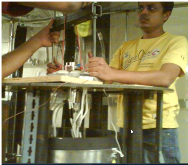
Figure 4-18 EEC motor being guided within the test rig
