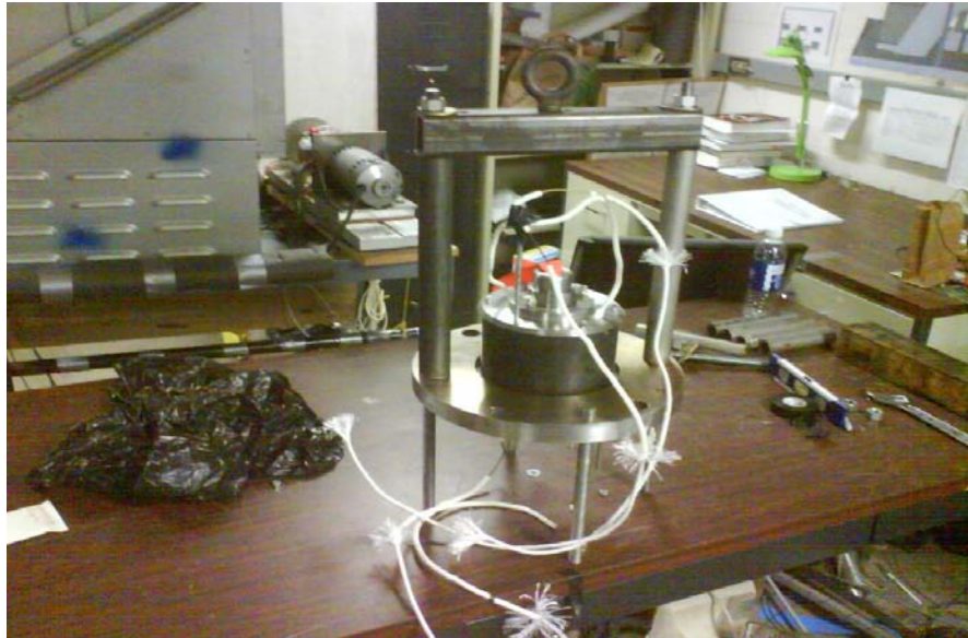
Figure 4-3 Specially designed and fabricated fixture for handling the thrust bearing
