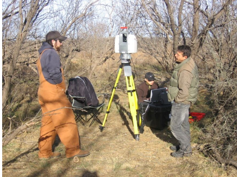
Figure 2. Terrestrial lidar system, Leica ScanStation2, in the field setting of this study.
