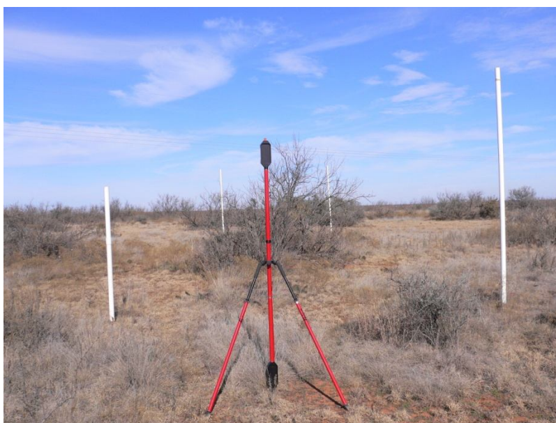
Figure 5. Scattered mesquite trees in a study plot (Plot U20) and a target (red) used for merging the two scans of a plot from opposite directions. The white PVC pipes were used to mark the boundary of a study plot.
