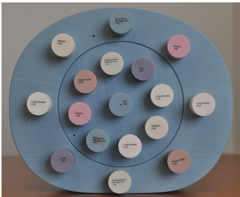
Fig. 2.6. CIRS 062 electron density phantom used for the CT number - electron density calibration. The phantom contains a two-part body, eight pairs of tissue equivalent inserts and a solid water insert. Tissue equivalent inserts include lung (exhale and inhale), adipose tissue, breast, liver, muscle, trabecular bone and dense bone.
