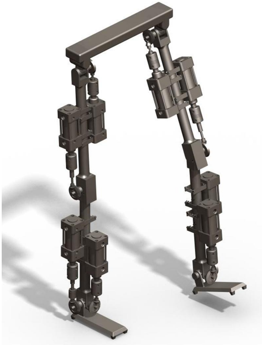
Figure 24: Rendered version of the final CAD model of the bipedal robot assembly
