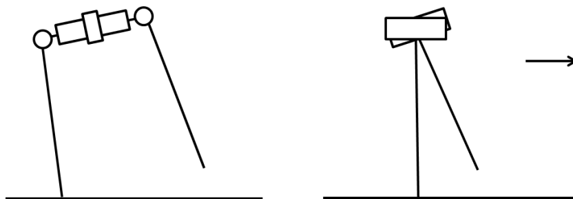
Figure 11: The purely “dynamic” model BIPER-3 with 4 DOF, Miura et al. [22]
