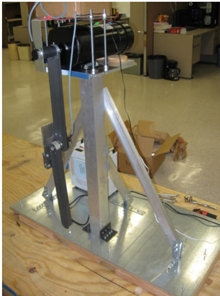
Figure 29: Snapshot of the physical setup of the double pendulum
