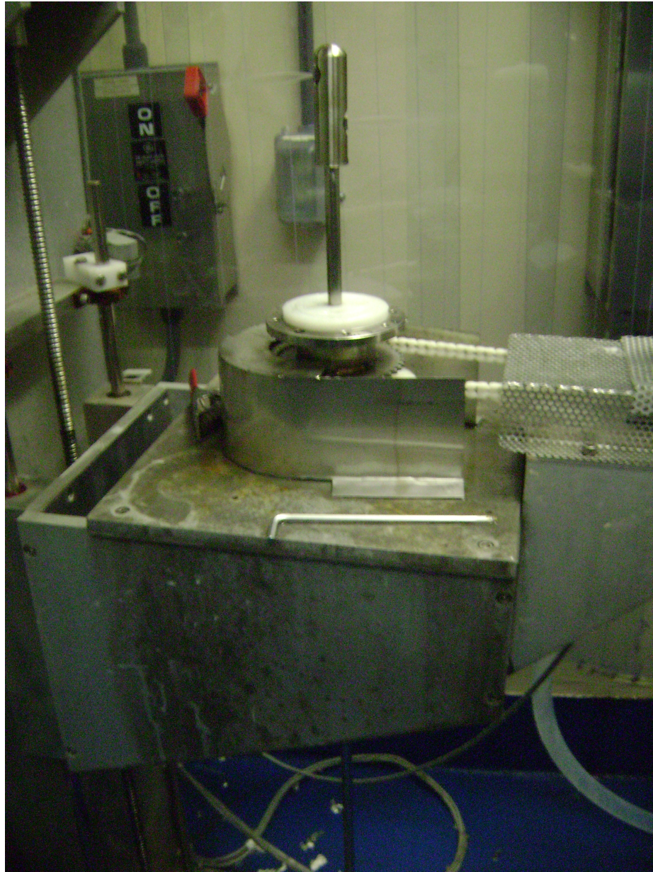
FIG. 31. High power rinsing device that moves up and down as the water jets rotate about the axis.
