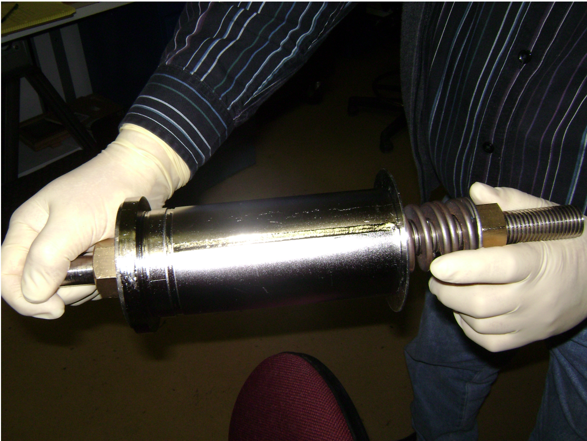
FIG. 32. Fixture is inserted through the parts to insure proper alignment. Pressure is applied through a spring loaded plate to keep the faces together and to handle the expansion and contraction of the metal during the welding process.
