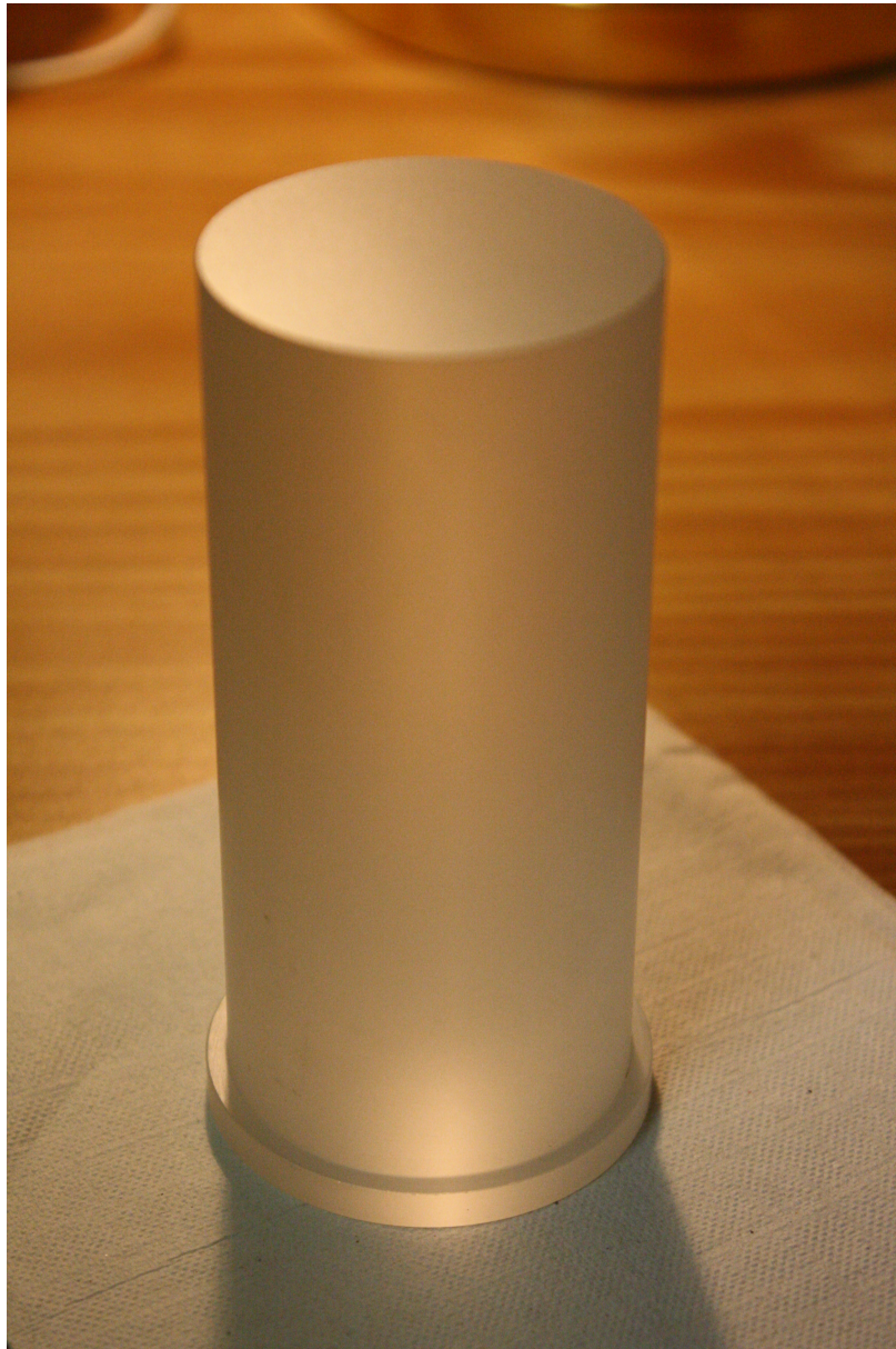
FIG. 36. The HEMEX single crystal to be used in the Sapphire Test Cavity is shown. Note that the dull color is due to the texture. The surface was ground and not polished. If the surface had been polished, it would have appeared as transparent glass. When placed in a liquid the crystal becomes essentially transparent.
