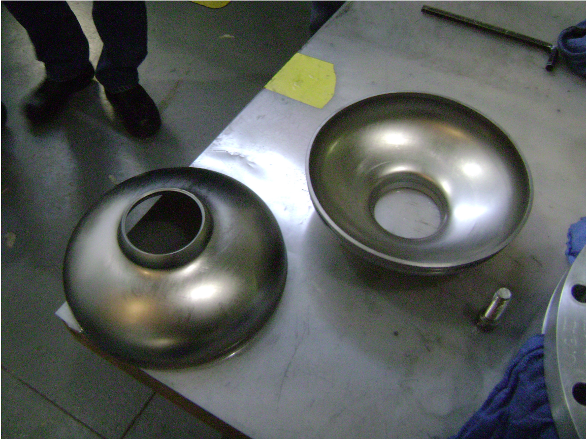
FIG. 30. Image of two half cells created directly after the pressing. Note that the center of the holes and lips of the iris are not symmetric. This asymmetry is most likely due to the material sliding in a preferential direction.
