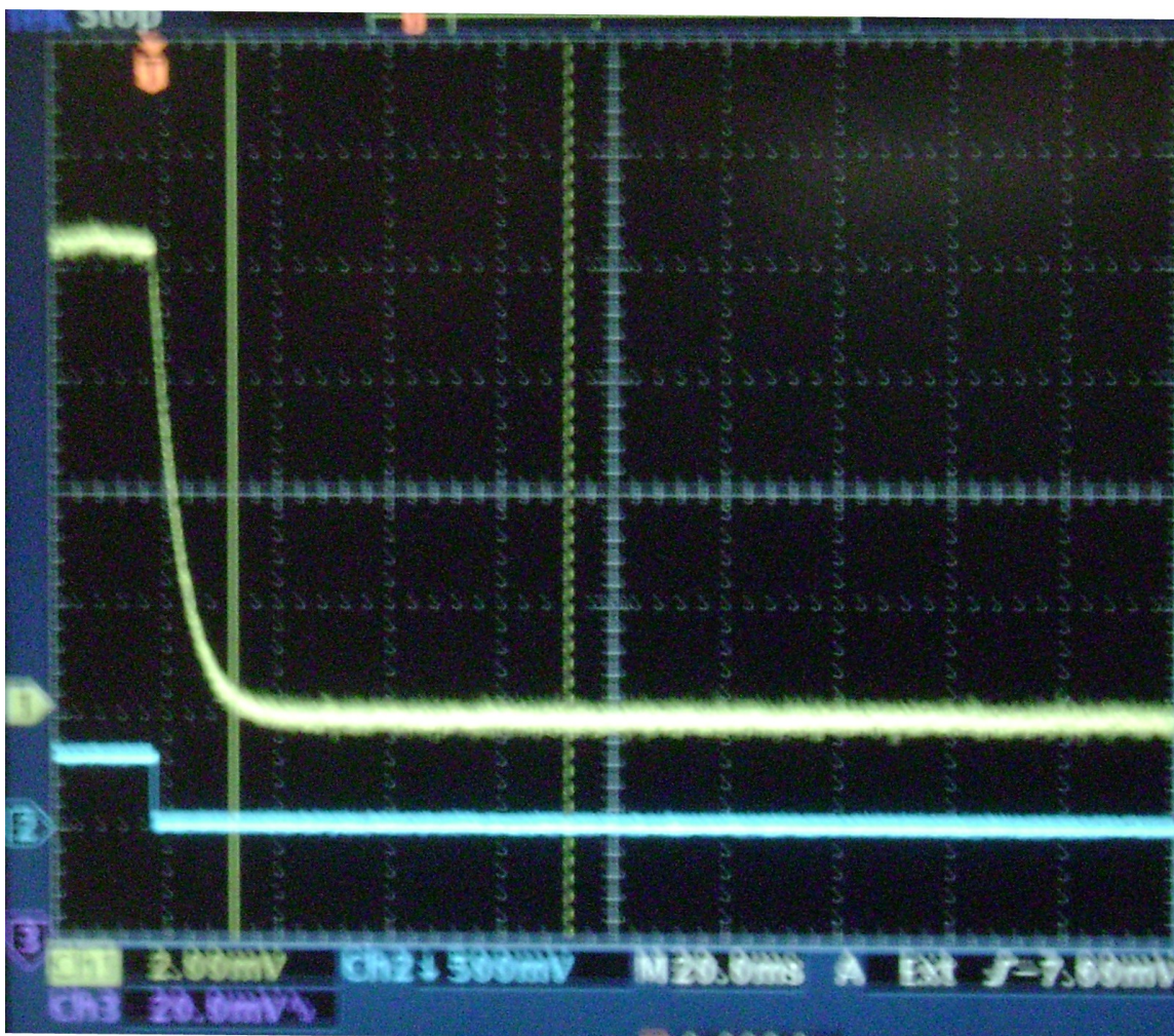
FIG. 66. The apex of the stored energy is captured during this measurement the left. Only the decay curve, the only slope changing line, was captured allowing the Lab View program to statistically calculate the decay time.
