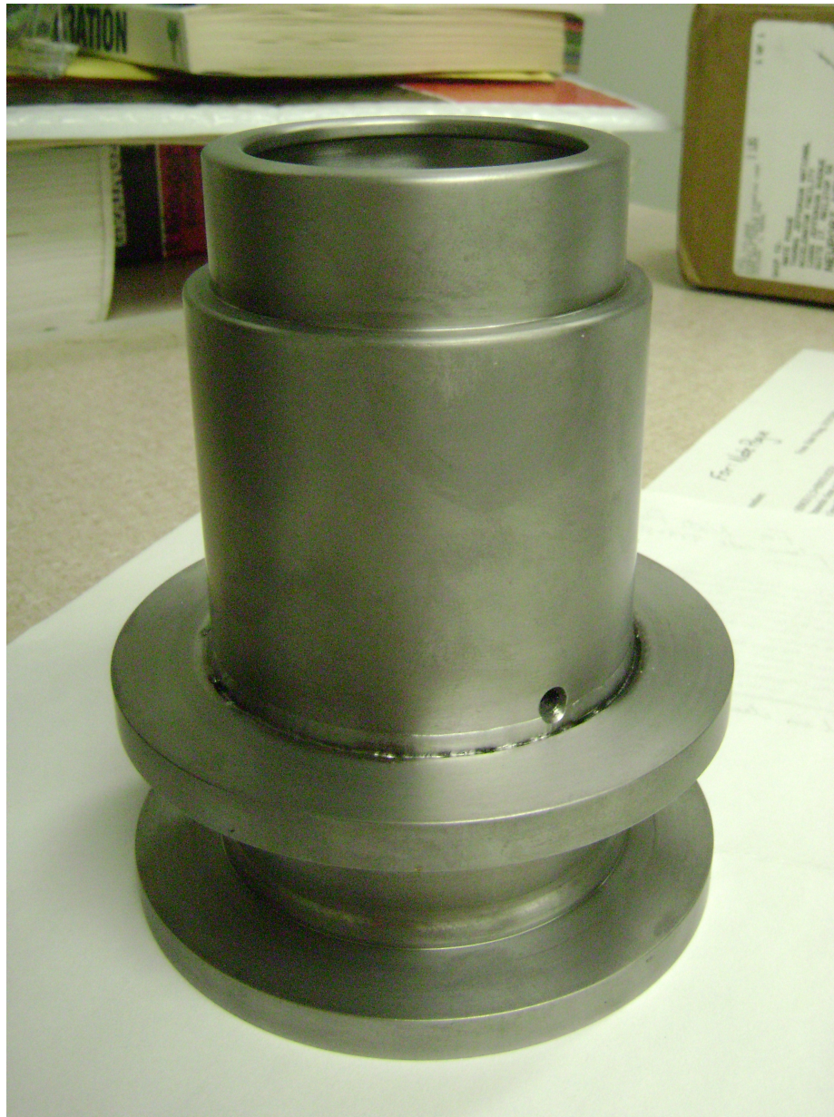
FIG. 37. The Niobium holding fixture is used to suspend the sapphire in the cavity. Holes are located in sides for evacuation of tube.
