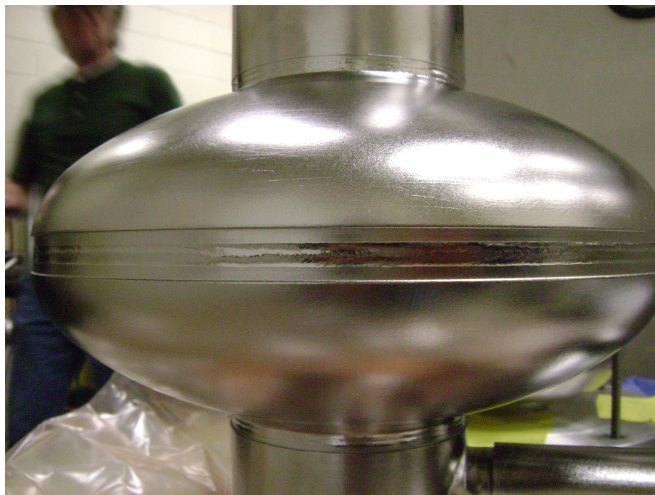
FIG. 35. The equator joint after e-beam welding.
