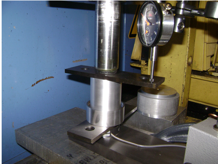
FIG. 41. This is the set-up for the indium seal test. Two parallels sandwich a sapphire placed in the holder with a backing plate and pushing bar placed on top of it. The entire fixture was then placed on top of a load cell, after which the entire contraption is put into a hydraulic press.
