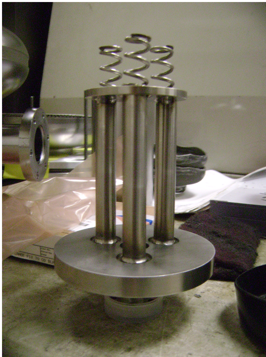
FIG. 39. This 316 stainless steel structure pushes down the backing plate with a large uniform load. It is attached to the top of the niobium holder, creating indium vacuum seal. It also serves as the means by which the thermometers are connected to the read out, via the electrical feed through at the top of the fixture.
