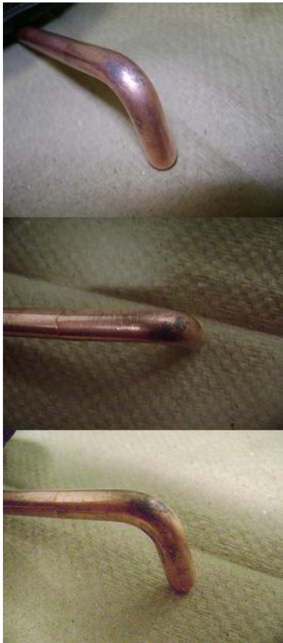
FIG. 60. Dark discoloration on copper may be proof that multipactoring was occurring on drive port antenna.
