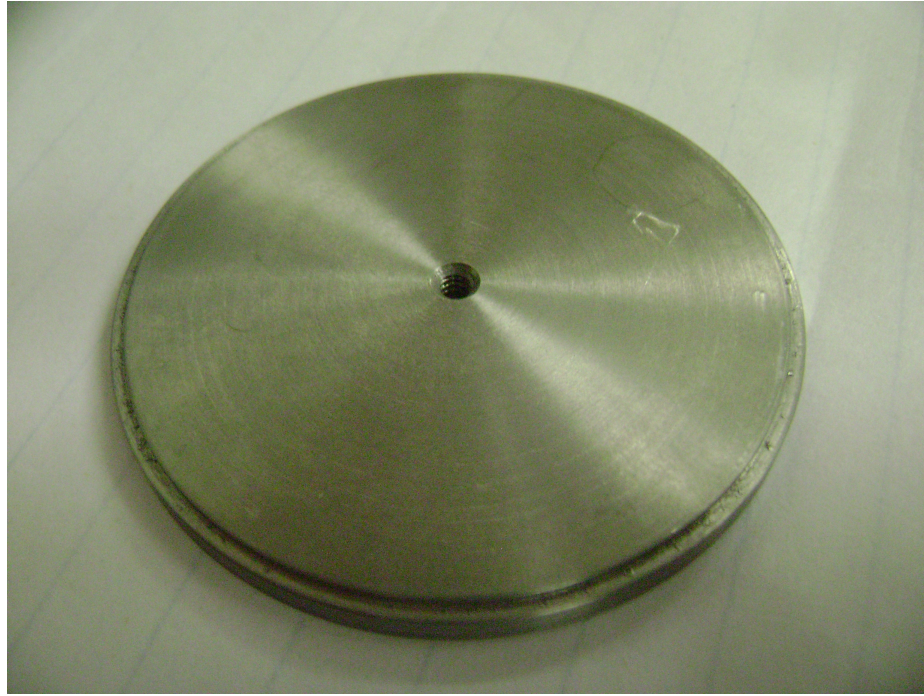
FIG. 38. The niobium backing plate has a groove on the circumference that has a .045 inch well that is recessed from the circular edge by .025 inches, giving a cross sectional area of .001125 square inches. The cross section of the indium wire is .001257 square inches, forcing the indium to flow between surfaces of the sapphire-sidewalls-backing plate intersection.
