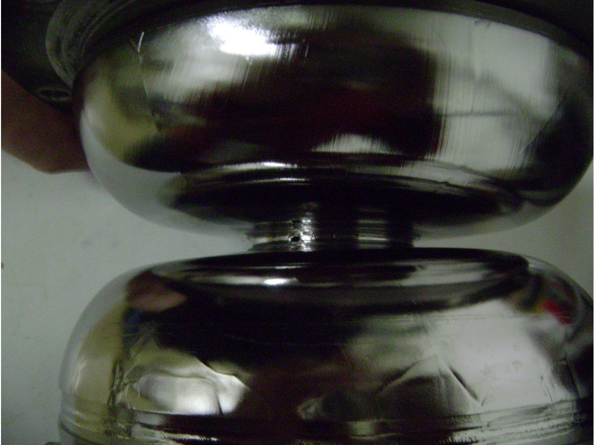
FIG. 34. Image of a hole created in the final iris of a 7-cell cavity during e-beam welding.
