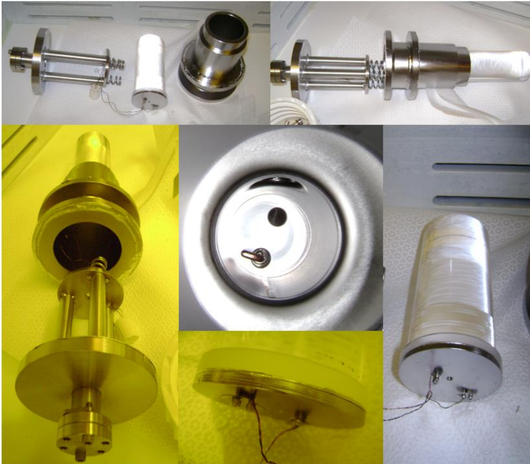
FIG. 79. Final state of dielectric test cavity. Upper left: interior parts of cavity laid out, note the dielectric feed through is not in the port because it was replaced with mesh on the last test allowing it to freely hanging inside the cavity. Upper Right: sapphire assembled with pusher plate slightly inserted into the holder. Lower Left: Assembly view. Middle: interior of the Niobium cavity. The side port is directly up and the hook antenna can be seen at the far end, pointing azimuthally as modeled. Lower Middle: Backing plate attached to the sapphire. Here Niobium marks can be seen on the crystal surface. Also looking at the resistor leads it can be seen that the gold lead is broken. Lower Right: Good thermal contact between the sapphire and backing plate is shown, the resistors are firmly mounted, and the surface of the sapphire is still extraordinarily clean. The streaks seen are the holes in the class 100 towels used as a clean barrier on the table below the sapphire.
