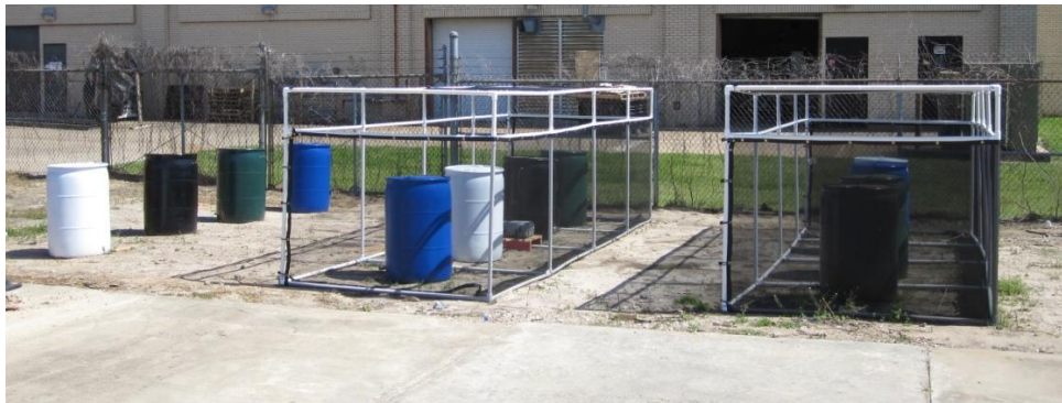
Figure 2. The research setup showing three blocks of shade treatments, each with four color treatments. The three blocks are (left to right): 0% shade, 30% shade, and 63% shade.
