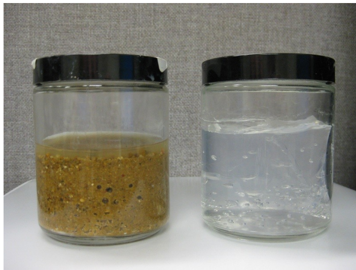
Fig. 4.6: Translucency of sandy soil (left) compared to Laponite gel (right)
