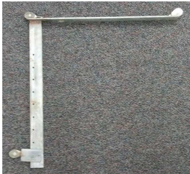
Fig. 4.3: Anchor line guidance system
