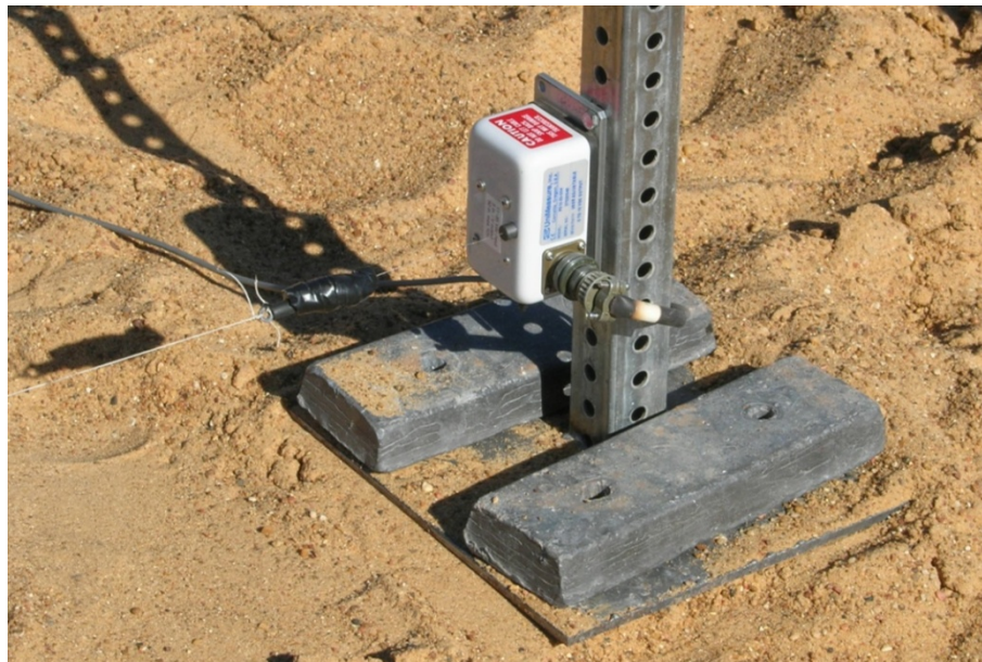
Figure D.5. Displacement measurement of static load test on a post for the impact test on a group of posts system in loose sand
