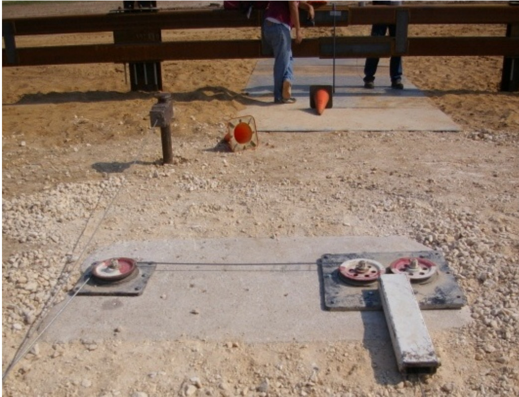
Figure 3.156. Vehicle guidance system for the full-scale test on group of posts
