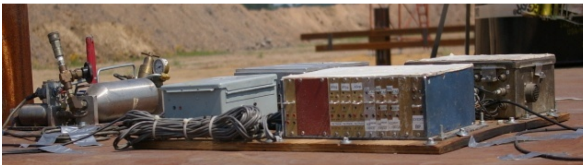
Figure 3.157. Accelerometers and data transmitter installed on the test vehicle
