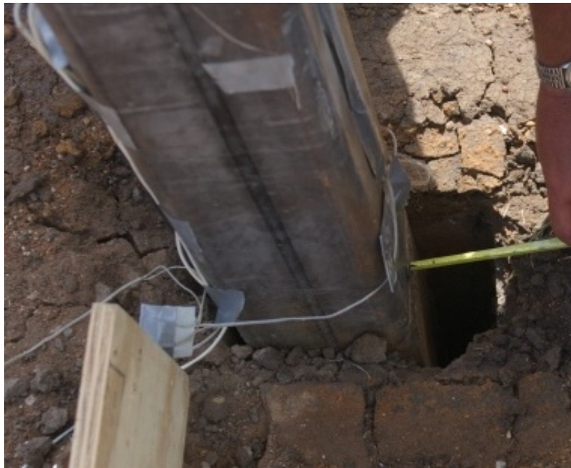
Figure 3.131. Displaced single post embedded in hard clay after impact test (B1)
