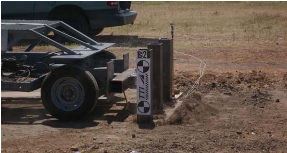
Figure 3.136. Bogie test on group of posts system embedded in stiff clay (B2)
