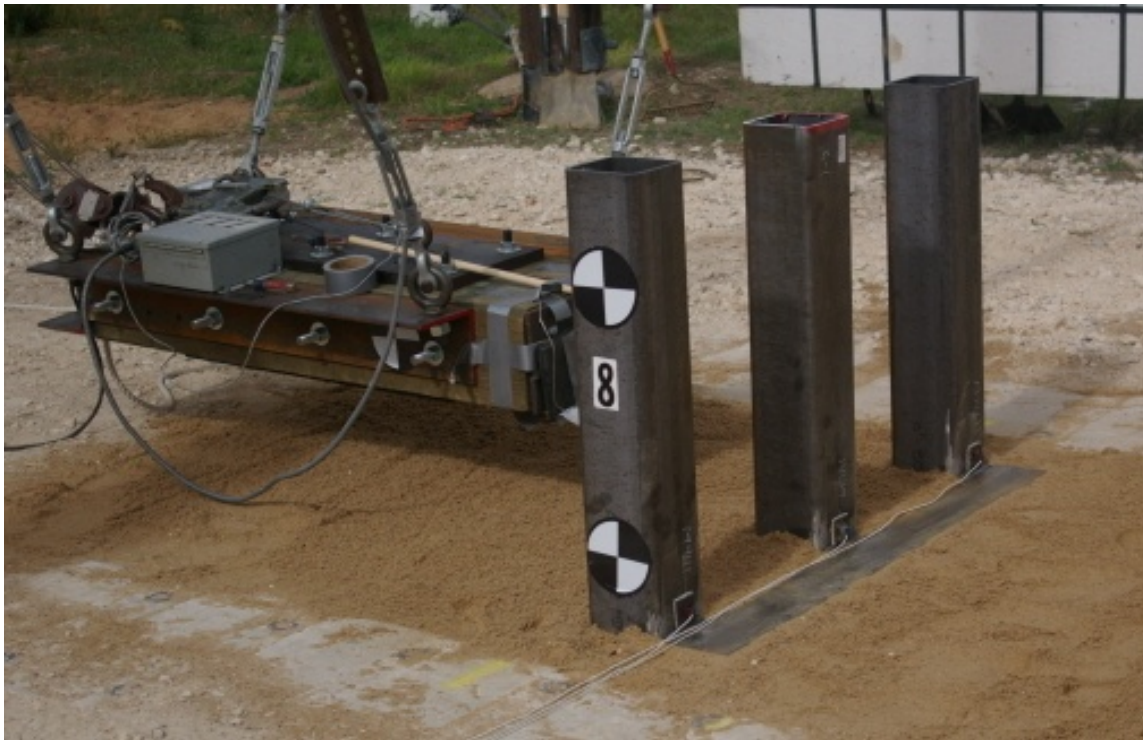
Figure 3.75. Pendulum test on group of posts system embedded in loose sand (P8)
