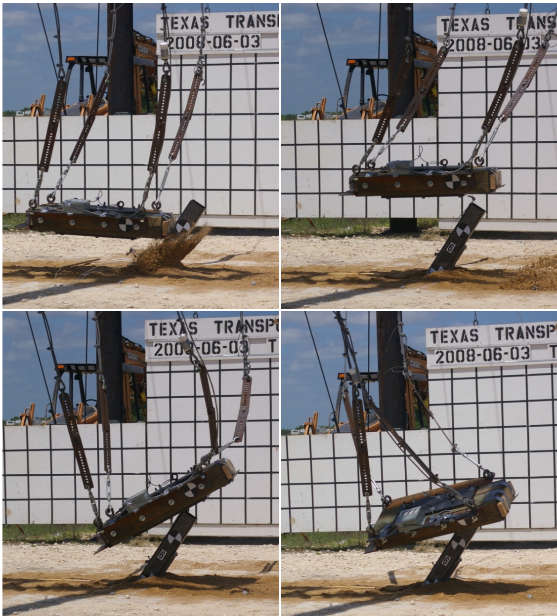
Figure C. 3. Pendulum test on a single post embedded in loose sand (P6)
