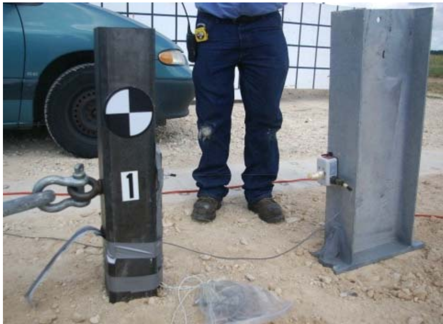
Figure 3.51. Displacement measuring system for static load test
