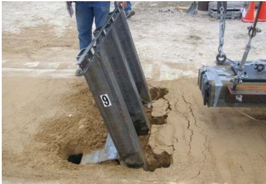
Figure 3.102. Displaced group of posts system embedded in loose sand after impact test (P9)
