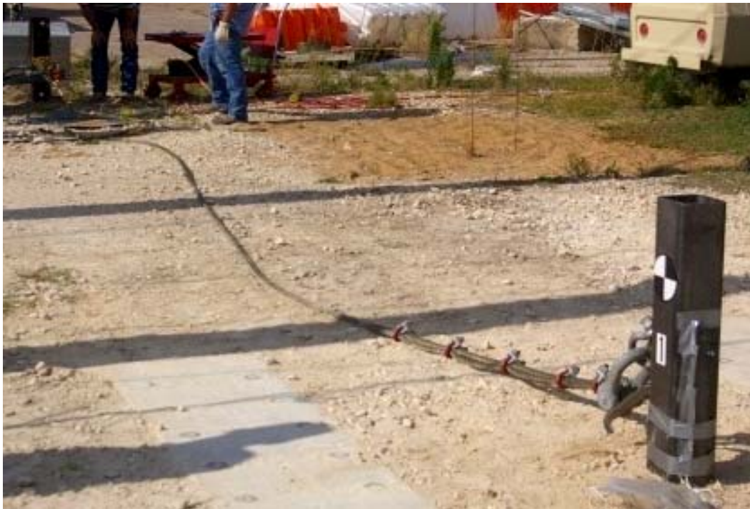
Figure 3.50. Pulling system for static lateral load test
