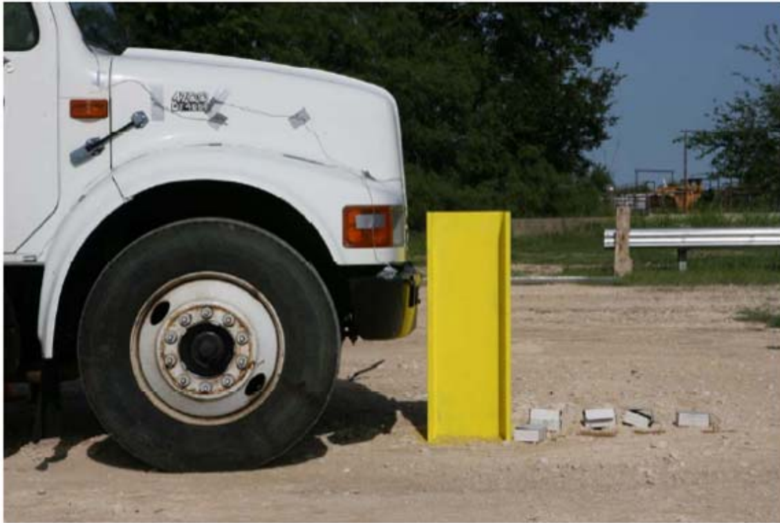
Figure 3.20. Full-scale M50 impact test on single post (Alberson et al. 2007)
