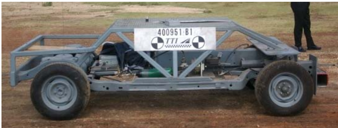
Figure 3.124. Bogie test with 900 kg (1990 lb) of mass used for the proposed tests
