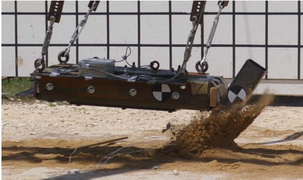
Figure 3.87. Pendulum test on single post embedded in loose sand (P6)
