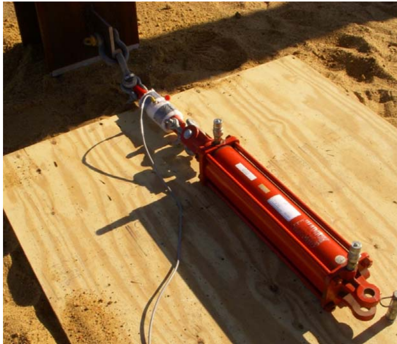
Figure D.4. Hydro Jack for static load test on a post for the impact test on a group of posts system in loose sand
