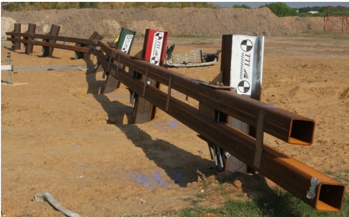
Figure 3.163. Deformed group of posts system after the impact
