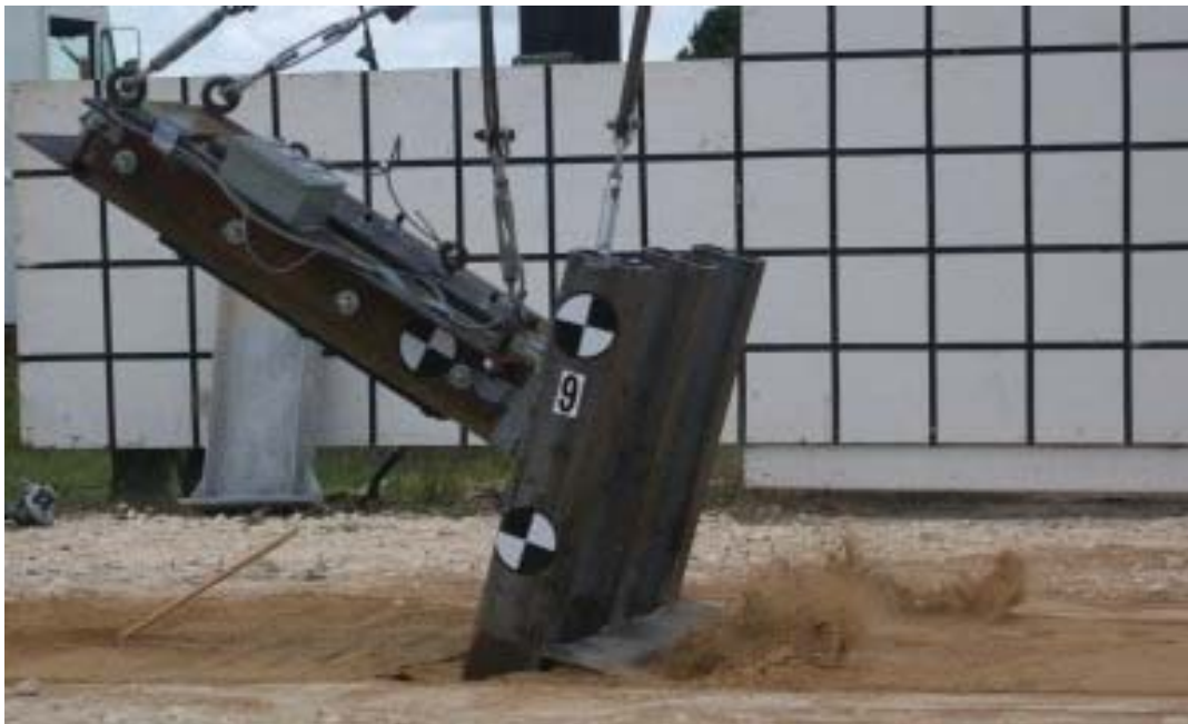
Figure 3.101. Pendulum test on group of posts system embedded in loose sand (P9)
