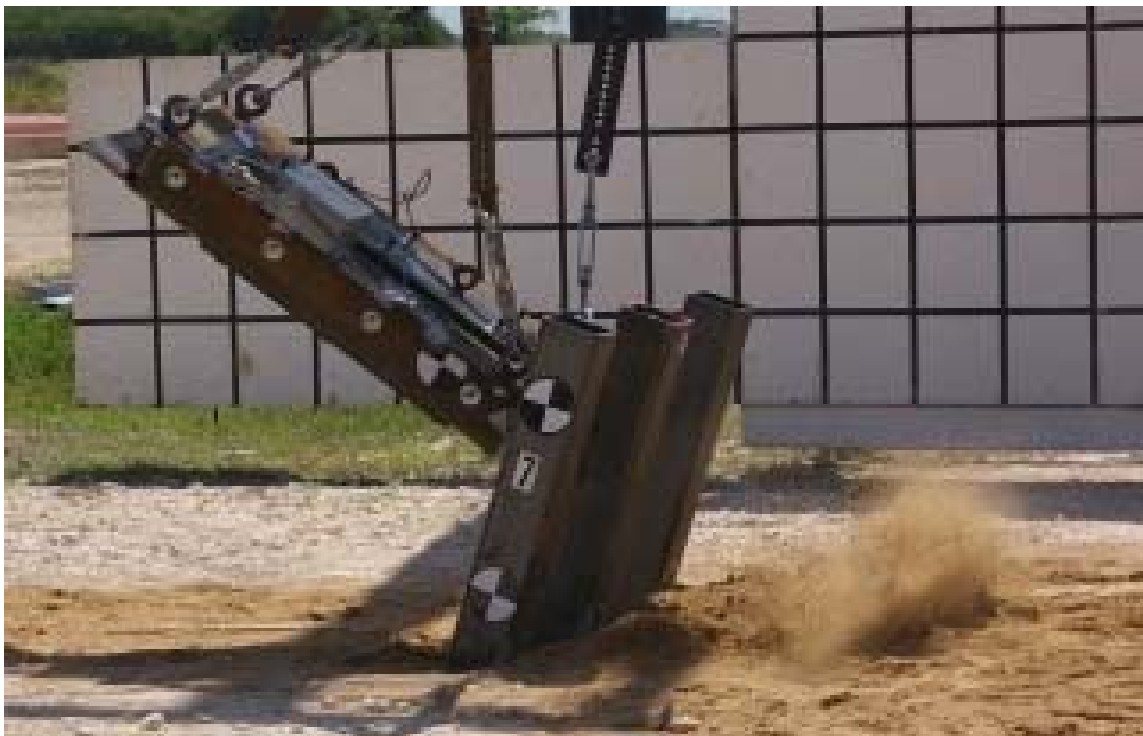
Figure 3.92. Pendulum test on group of posts system embedded in loose sand (P7)
