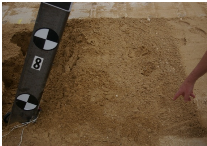
Figure 3.97. Displaced soil after impact test (P8)
