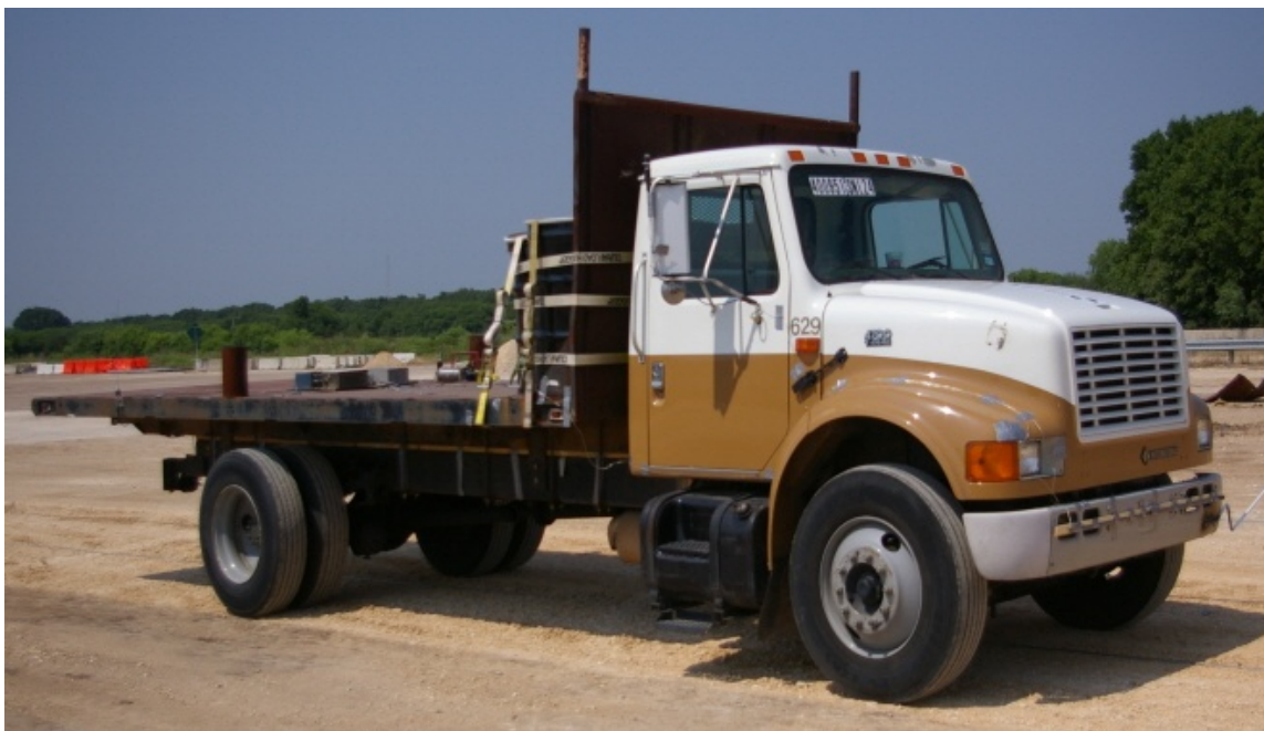
Figure 3.155. Test vehicle for the M50 impact on the group of posts system
