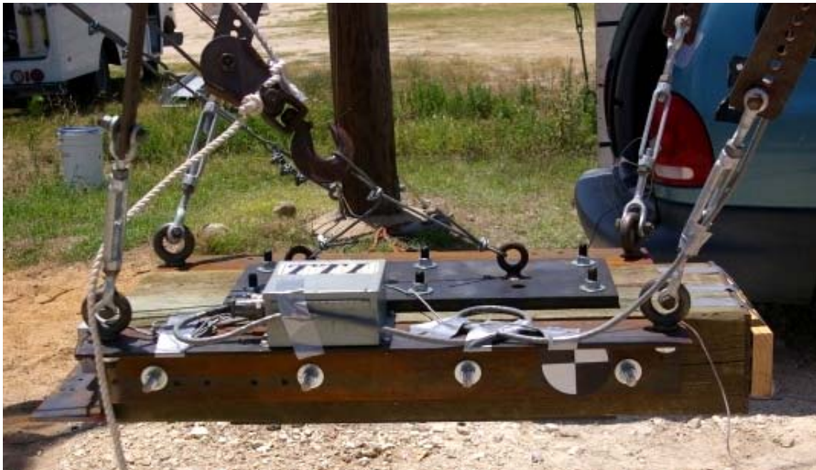
Figure 3.71. Small pendulum test on single post embedded in crushed limestone
