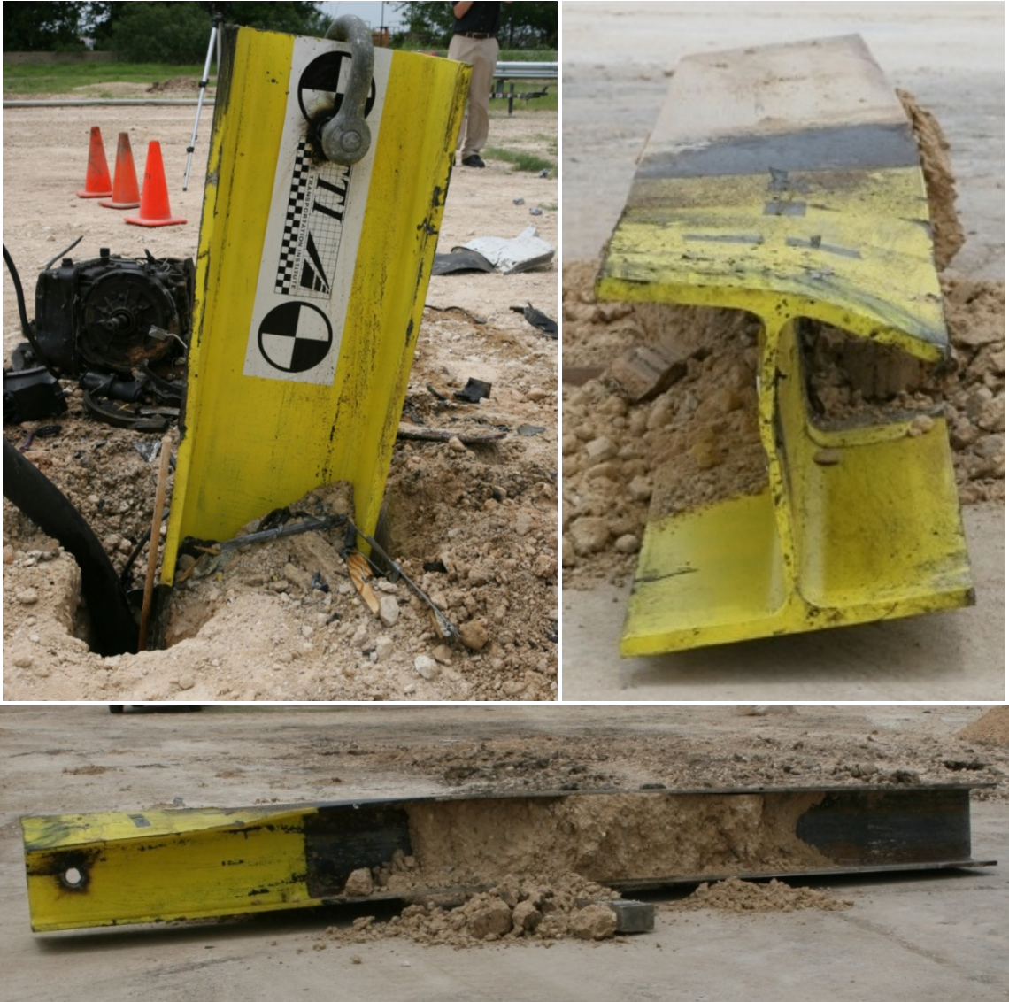
Figure 3.28. The single post after the impact (Alberson et al. 2007)
