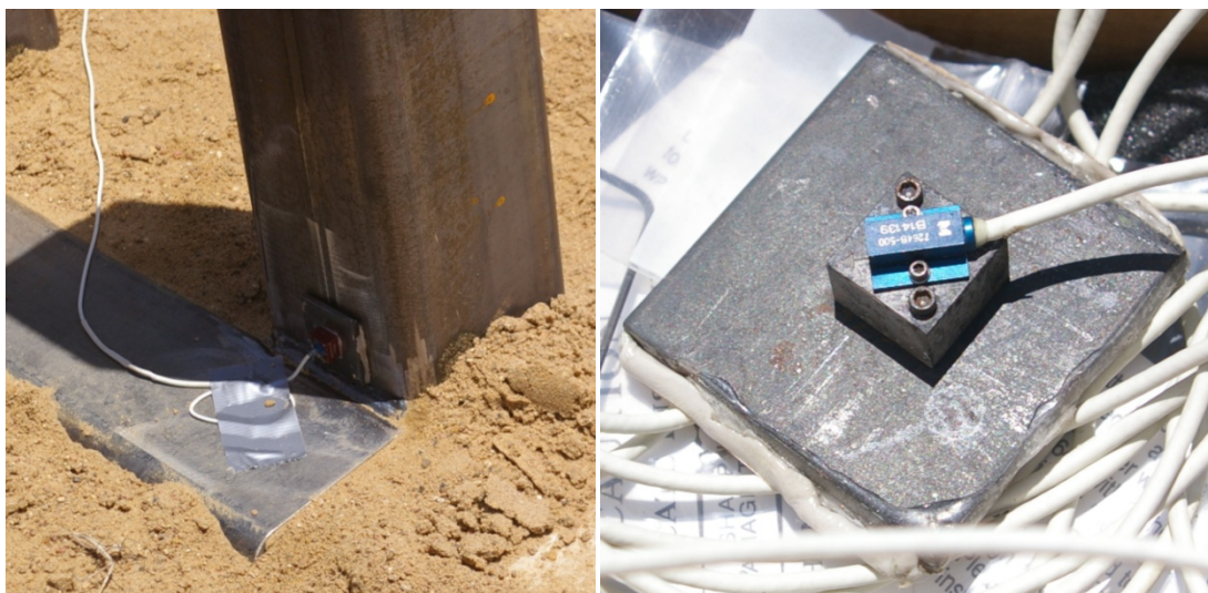
Figure C. 5. Accelerometer attached on a post system during pendulum test
