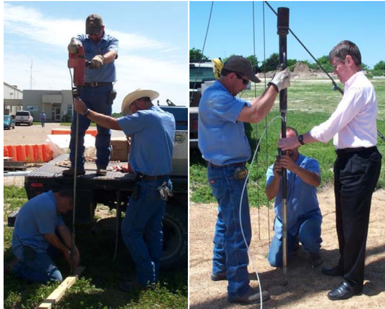
Figure A. 2. Preparing a borehole and lowering the probe by driving
