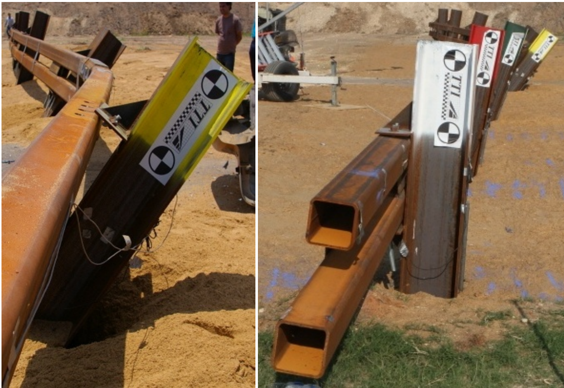
Figure 3.164. Broken connection of the two center posts
