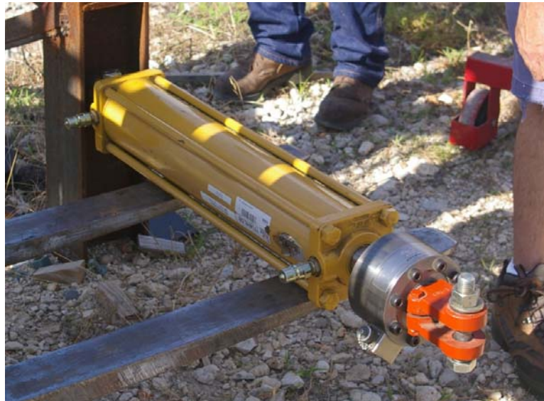
Figure C. 1. Hydro Jack for static load test on posts for the model test
