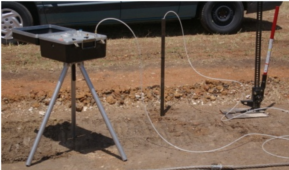
Figure 3.15. Pressuremeter test for hard clay for the bogie tests
