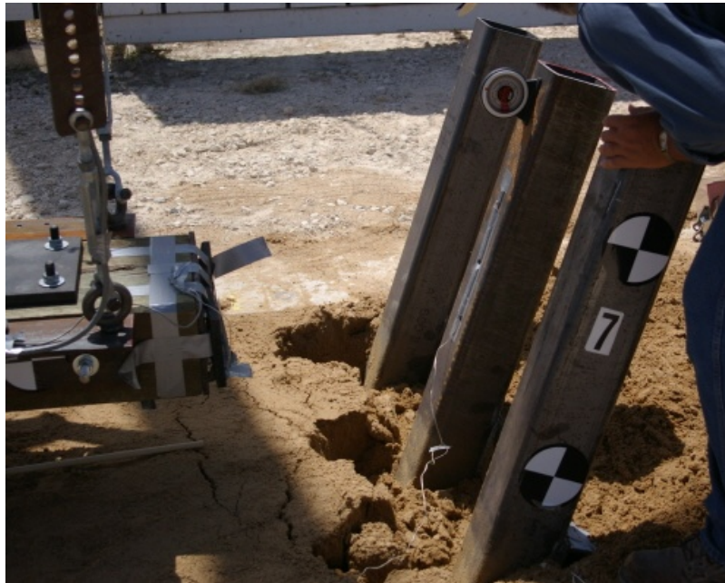
Figure 3.93. Displaced group of posts system embedded in loose sand after impact test (P7)
