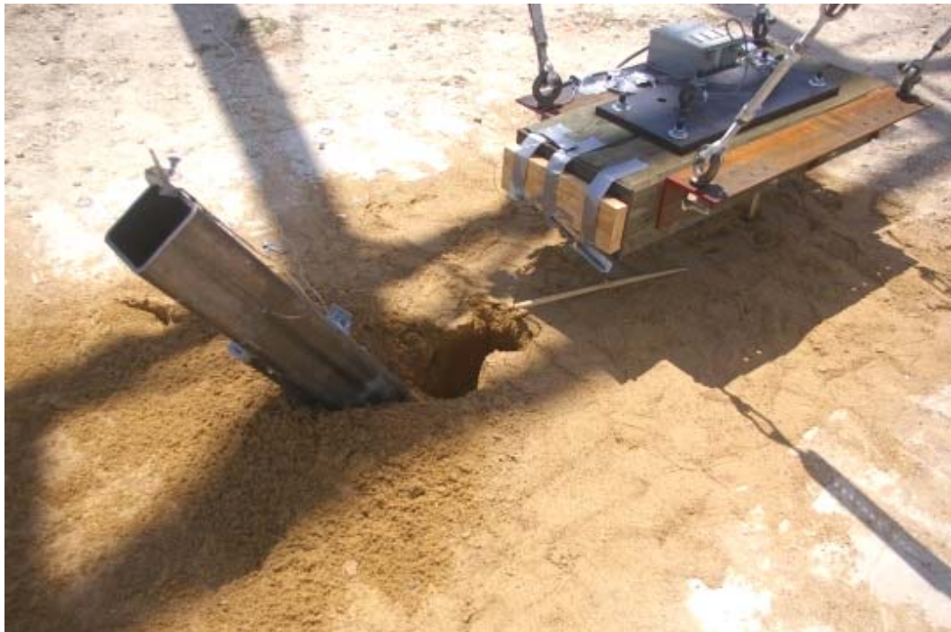
Figure 3.88. Displaced single post embedded in loose sand after impact test (P6)
