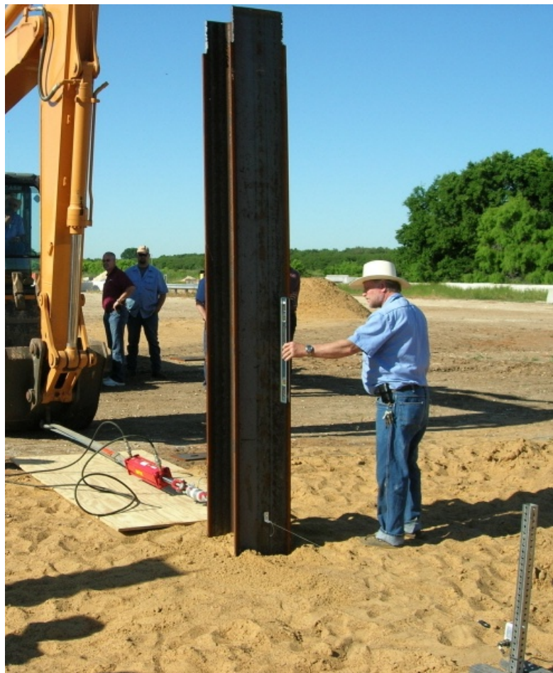
Figure 3.154. Static test on the single driven in loose sand ditch
