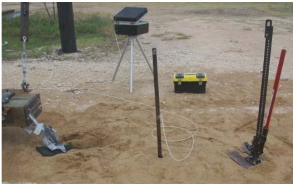
Figure 3.10. PENCEL pressuremeter test on the loose sand
