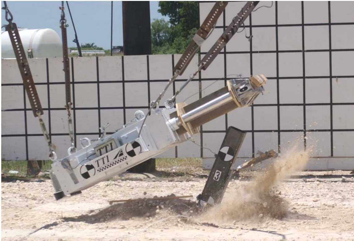
Figure 3.43. Model test using a pendulum with 860 kg of mass
