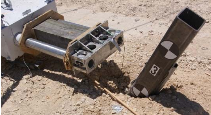
Figure 3.62. Deformed single post after pendulum test (P3)
