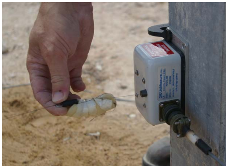
Figure C. 2. Displacement measurement of static load test on posts for the model test
