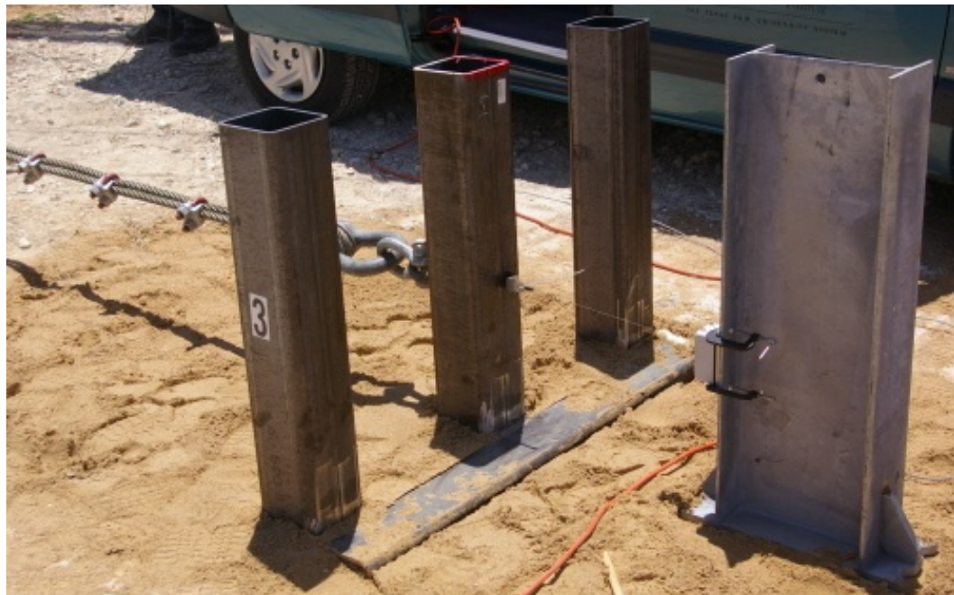
Figure 3.74. Instrumentations of the lateral static test (S3)
