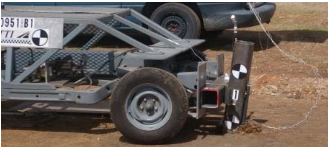
Figure 3.130. Bogie test on single post embedded in stiff clay (B1)
