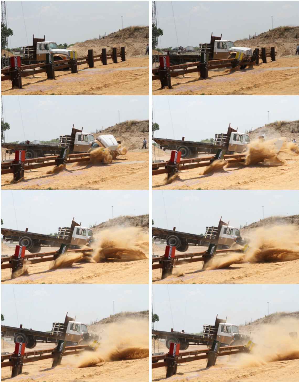
Figure D.8. Sequential photographs for the impact test on group of posts system
