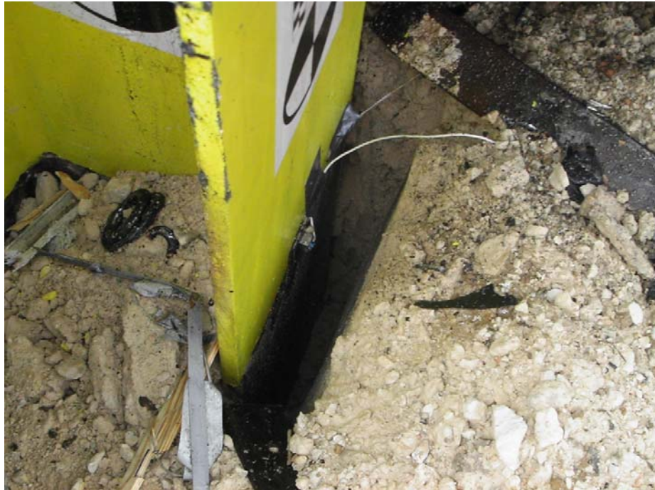
Figure B. 5. Soil deformation behind the post after the impact test
