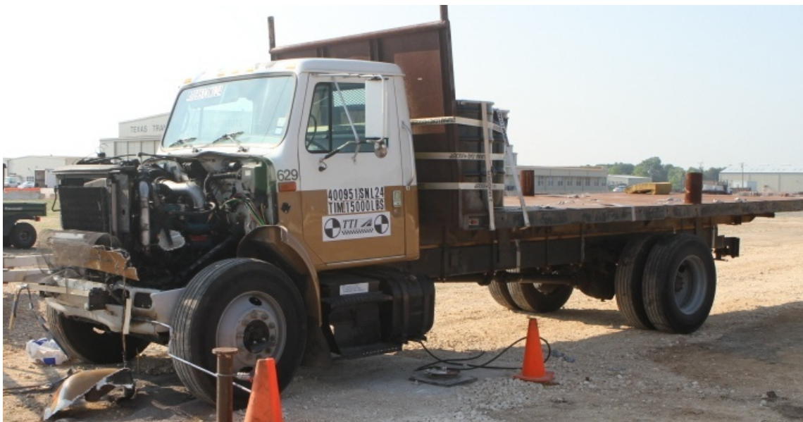
Figure 3.165. Deformed vehicle after the impact on the group of posts system
