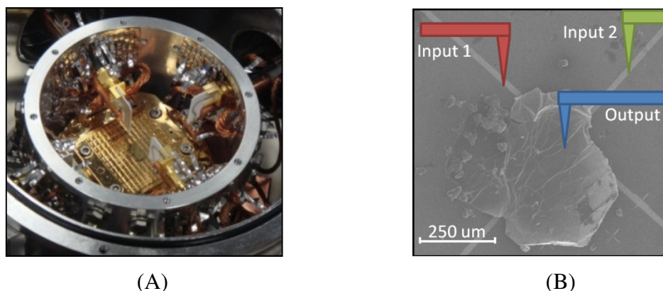
Fig. 71. (A) Four probe station chamber; each probe tip has a 3 \mu\text{m} diameter. (B) Fabricated device, a graphene sample of approximately six layers covers the gaps, two electrical signals are applied from the bottom of graphene using a pair of electrodes and the output is recovered from the top of the graphene sample.
