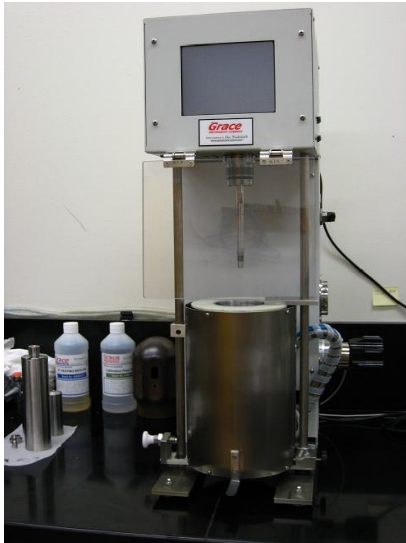
Fig. B.1—The photo of HPHT viscometer M5600.
