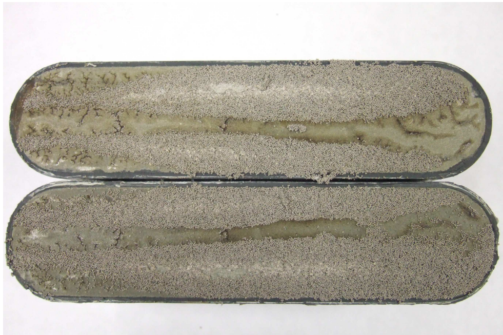
Fig. 3.9 Proppant placement with a channel in the middle
