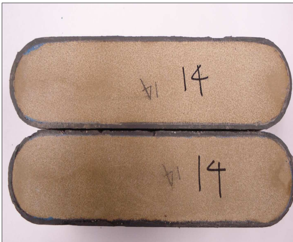
Fig. 3.17 Common indentation marks over cores surface after proppant was removed
