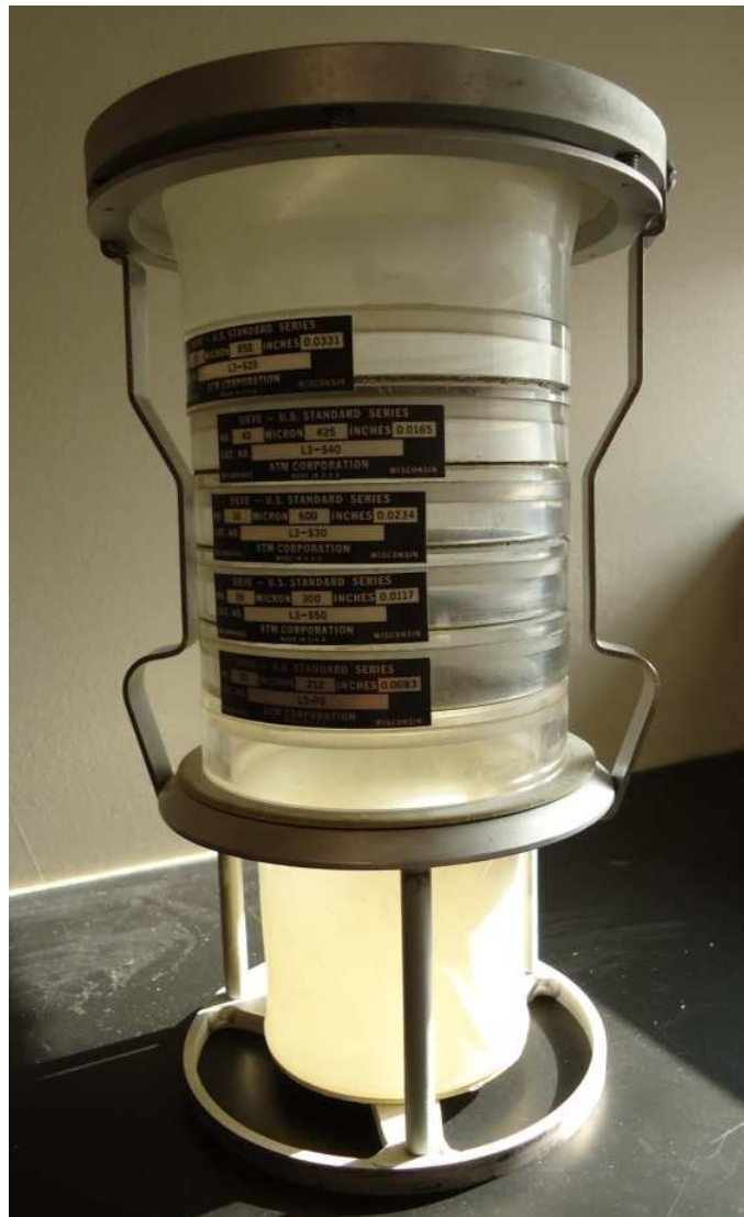
Fig. 2.16 Final assembly of the sieve analysis equipment
