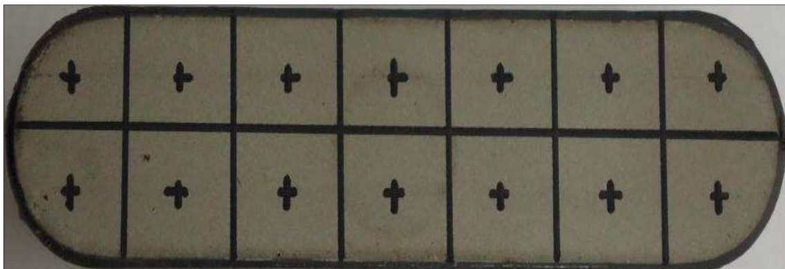
Fig. 2.15 Core surface with the points position for the embedment pressure test
