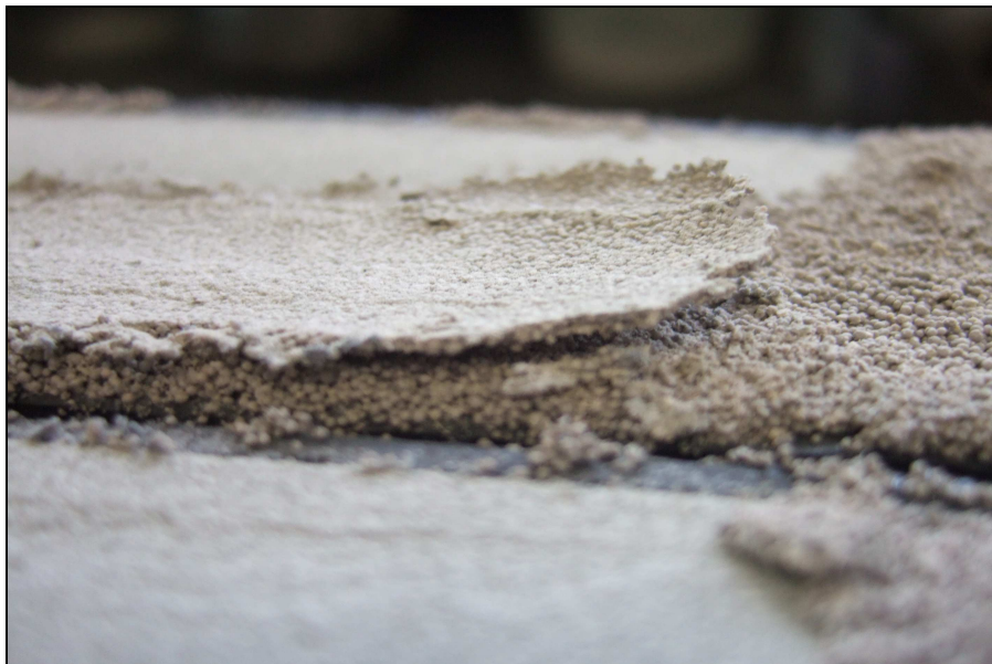
Fig. 3.16 Enlargement of the scale formed by proppant, fines, and dried polymer over the core surface
