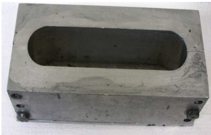
Fig. 2.8 Stainless steel mold used to prepare the cores
