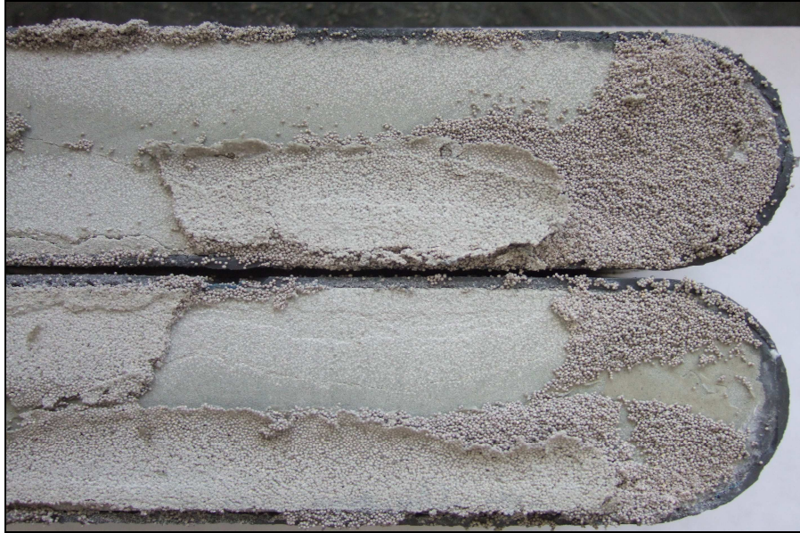
Fig. 3.15 Scale formed by proppant, fines, and dried polymer over the core surface
