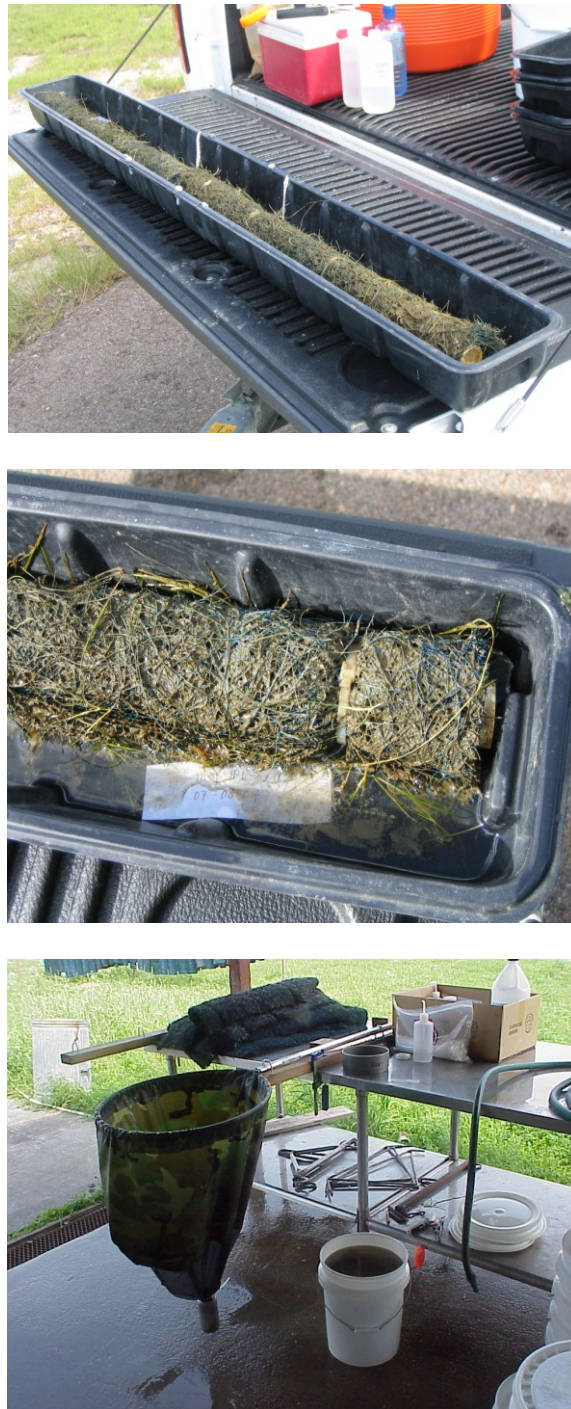
Fig. 2-4. Megalopal settlement collectors post-deployment. Upon retrieval, collectors were placed into trays and transported to land (top and middle). Filters were removed, placed in buckets filled with freshwater, and thoroughly washed to remove all organisms (bottom).
