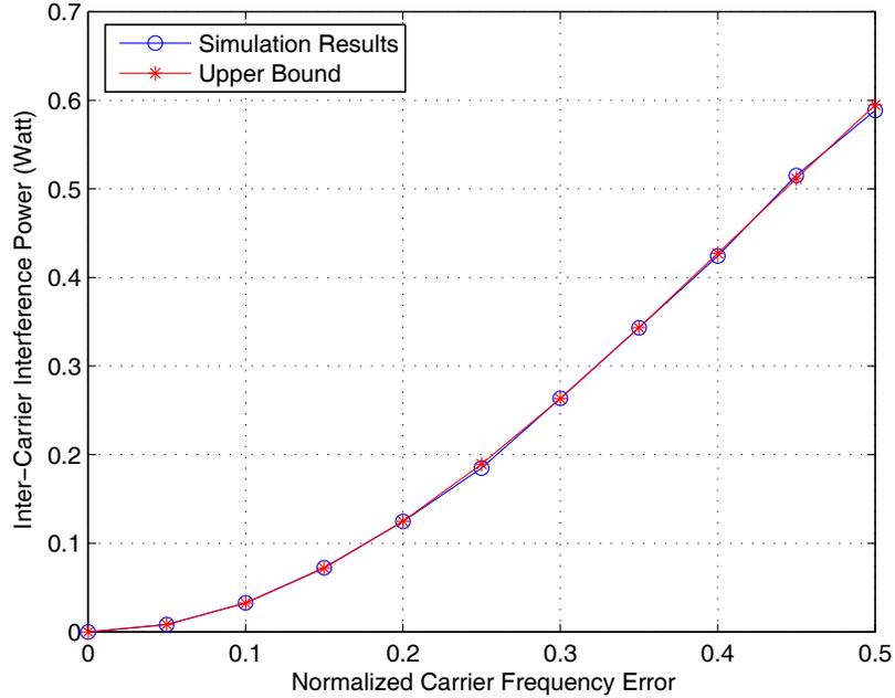
Fig. 4. ICI caused by carrier frequency offset.
