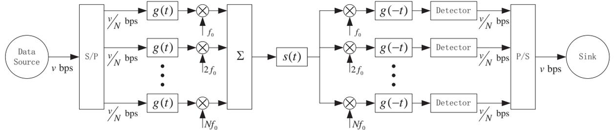
Fig. 1. A simplified block diagram of OFDM.
