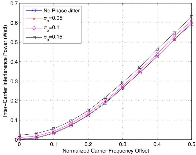
Fig. 5. ICI caused by carrier synchronization imperfection.
