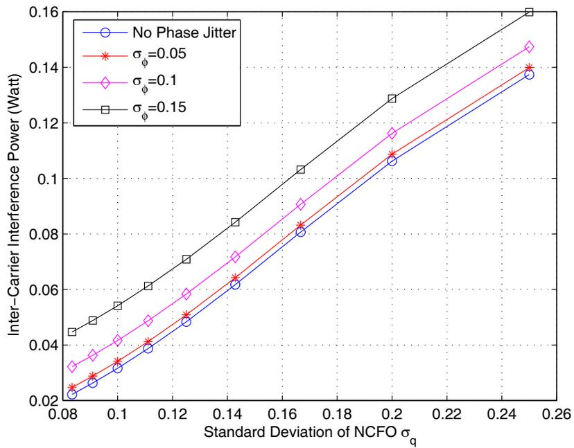
Fig. 6. ICI caused by carrier synchronization errors.
