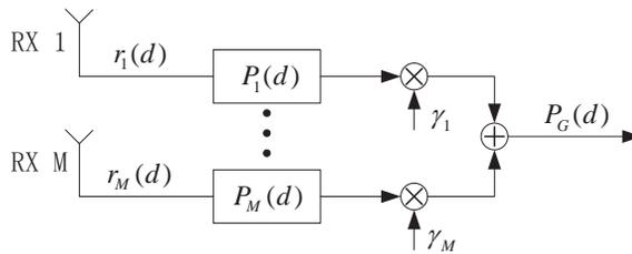
Fig. 13. Exploitation of receive diversity for synchronization.
