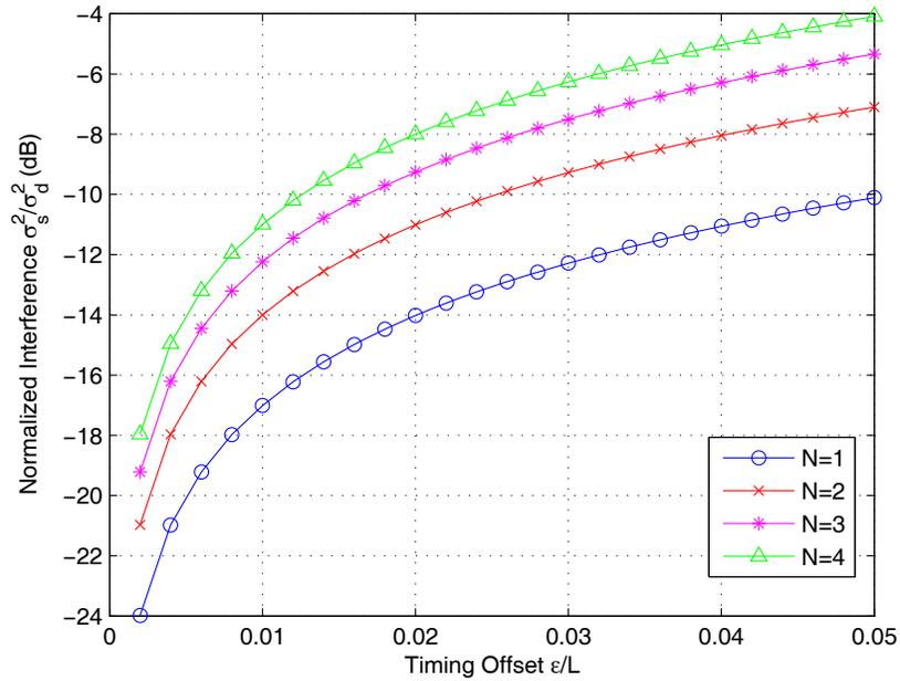
Fig. 10. Power of interference due to timing offset.
