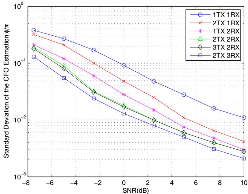
Fig. 16. Standard deviation of the CFO estimation.
