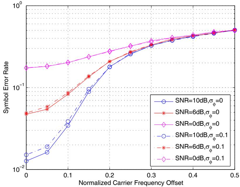
Fig. 8. Symbol error rates with imperfect synchronization.
