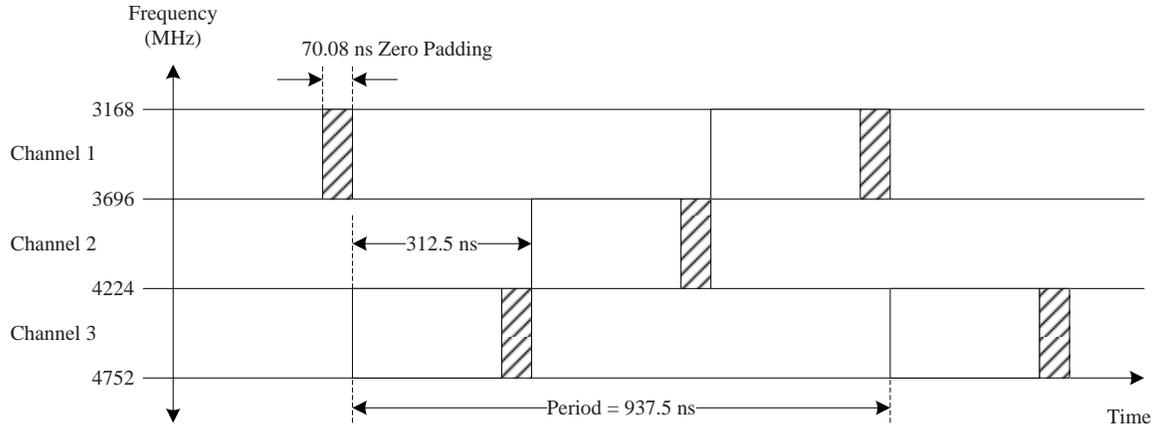
Fig. 2. Signaling diagram of the MB-OFDM system.
