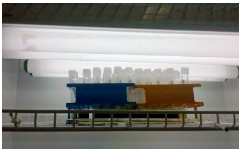
Figure 4-3. Experimental conditions for açai oil fractions. Oils were placed 10 cm directly under four fluorescent bulbs (10,000 lux) for 20 days.
