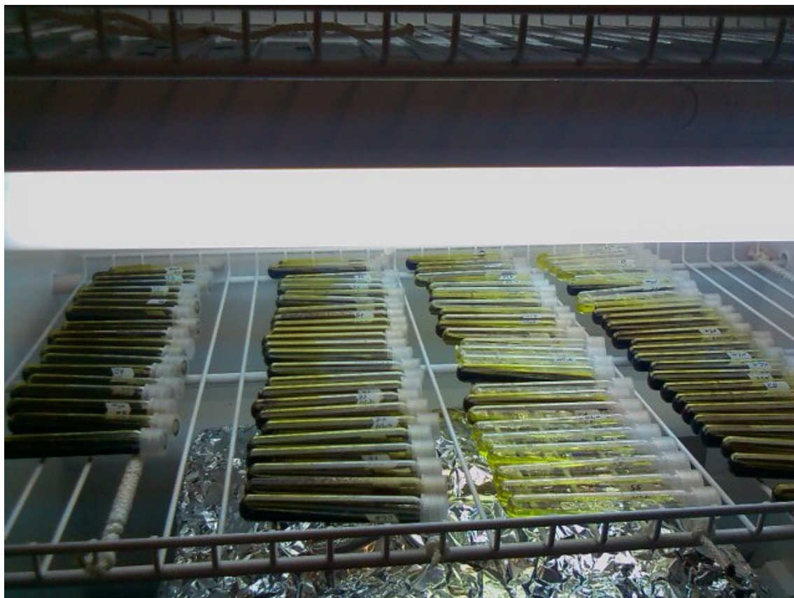
Figure 3-1. Experimental set-up for oils exposed to light for 25 days. Oils were placed 10cm directly under four fluorescent lights (10,000 lux).
