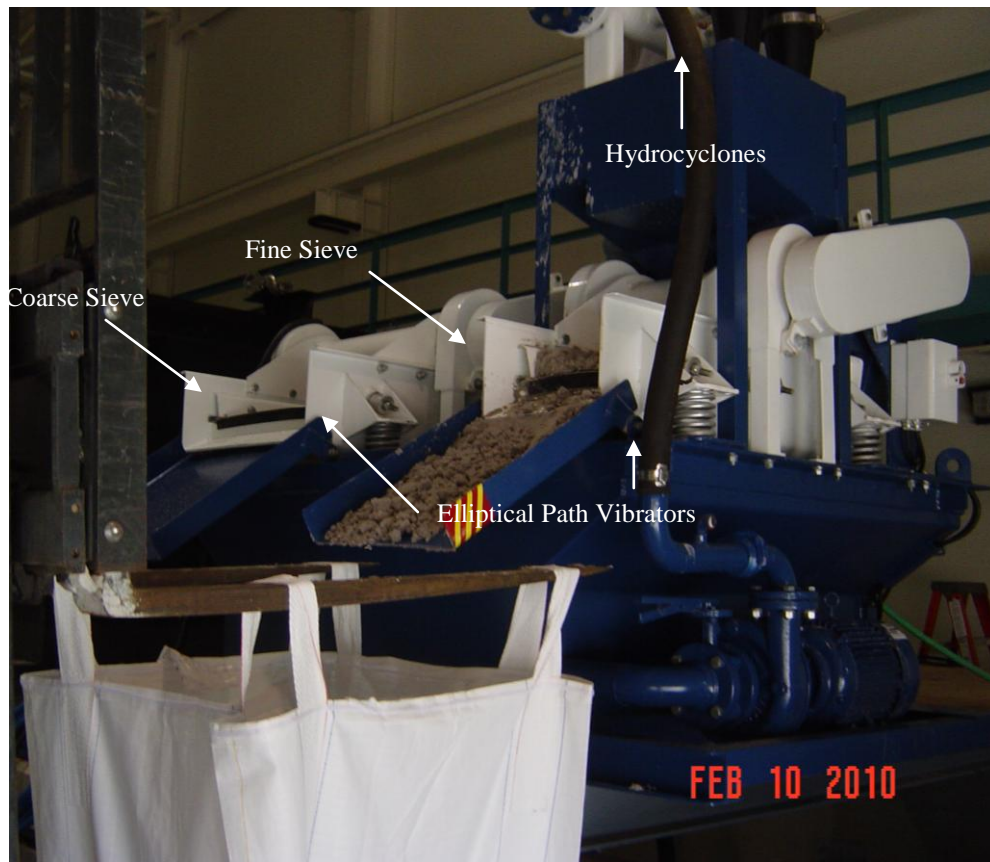
Figure 16. Sand Separation System in Operation
