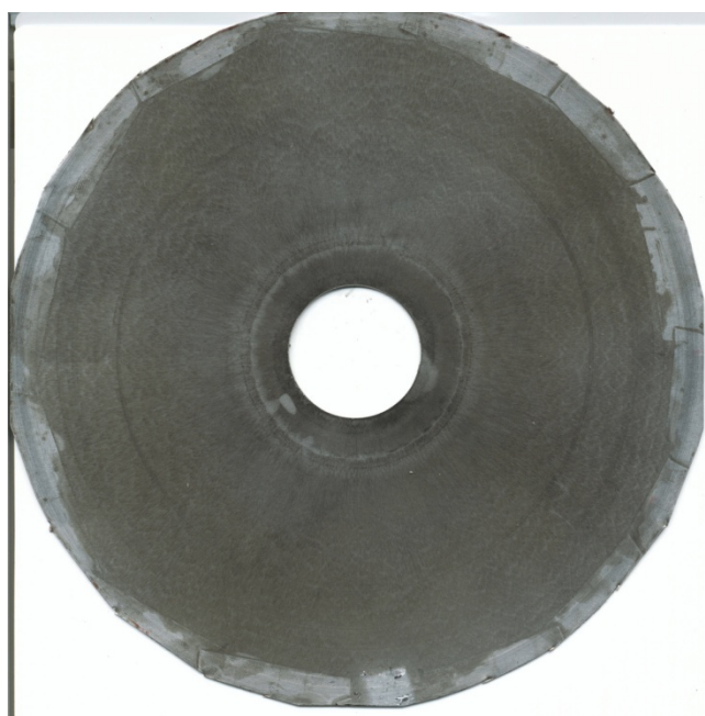
Figure B-5 Go. Run 240. 13.7 mm spacer. C_2H_2+4 O_2 . w/\lambda = 5.02 . Back wall.
