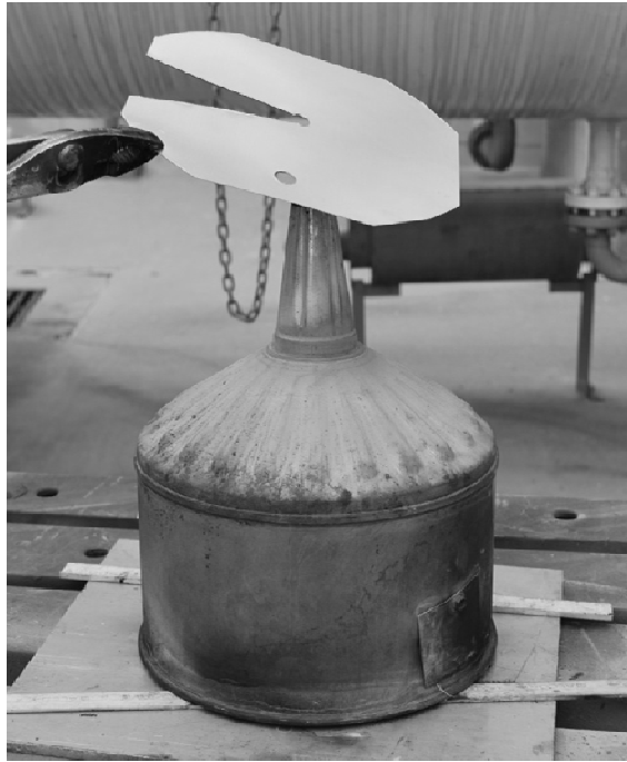
Figure 31 Second method attempted to create high-quality soot foils. This method did not yield repeatable results.
