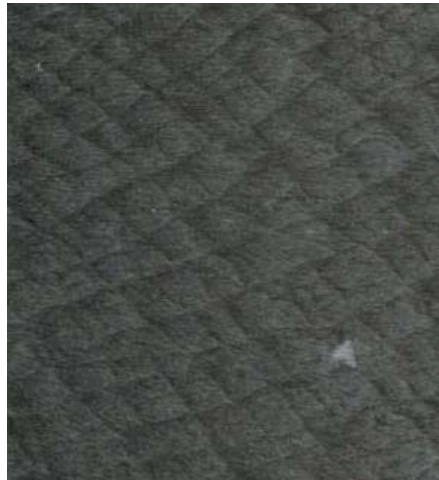
Figure 5 Experimental record of detonation wave cellular structure from the present study.
