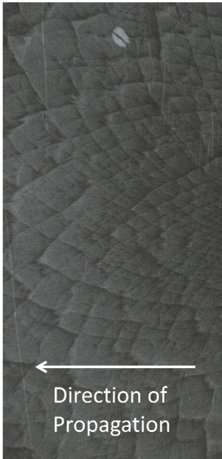
Figure 7 Experimental record of cellular structure for a diverging detonation wave from the present study. The cells grow larger as the detonation propagates radially outwards.
