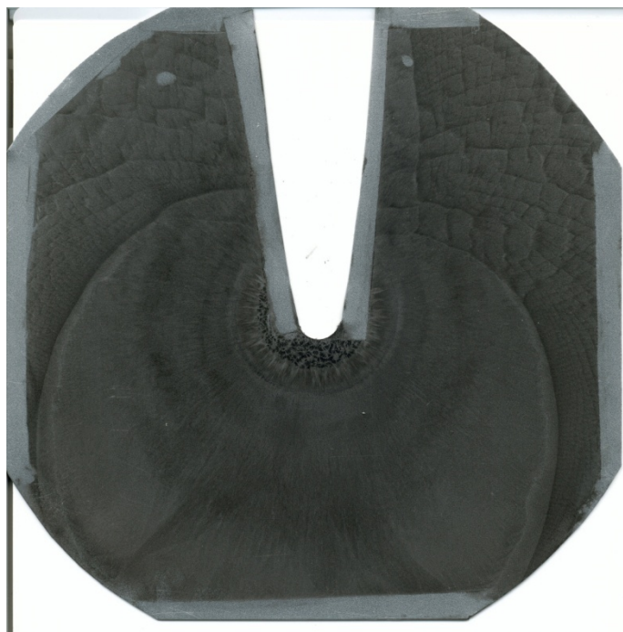
Figure B-21 Go. Run 283. 4.175 mm spacer. C_2H_2+2.5 O_2 . w/\lambda = 1.15 .
