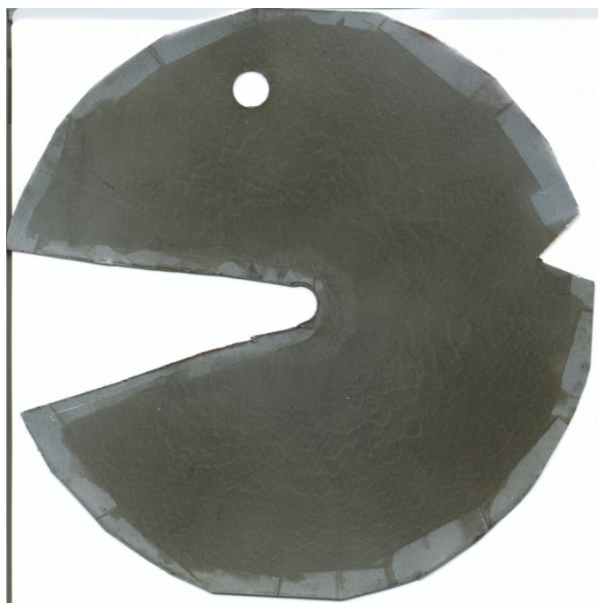
Figure B-4 Go. Run 240. 13.7 mm spacer. C_2H_2+4 O_2 . w/\lambda = 5.02 . Front wall.
