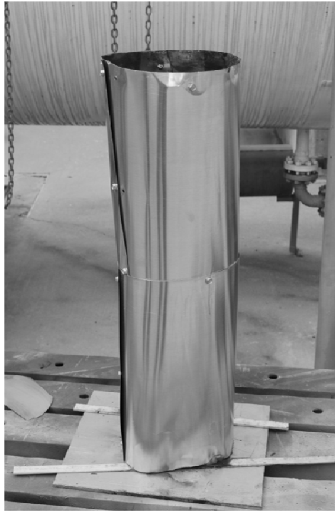
Figure 32 Chimney used in final method to produce soot foils. This method produced high-quality, repeatable results.
