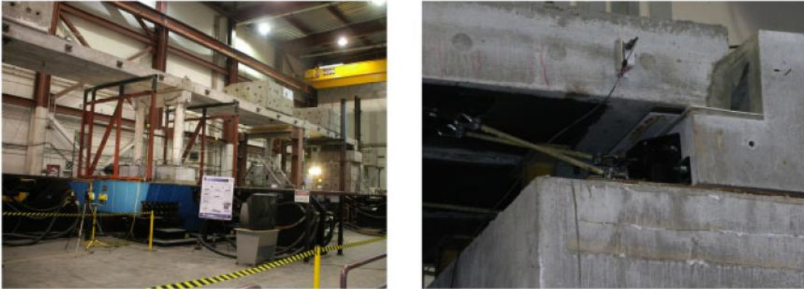
Figure 2-11 Experimental test setup and SMA restrainer (Padgett et al. , 2009)
