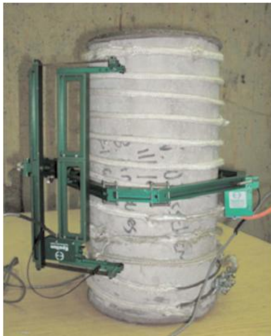
Figure 2-12 Concrete specimen with SMA spirals (Andrawes et al. , 2010)
