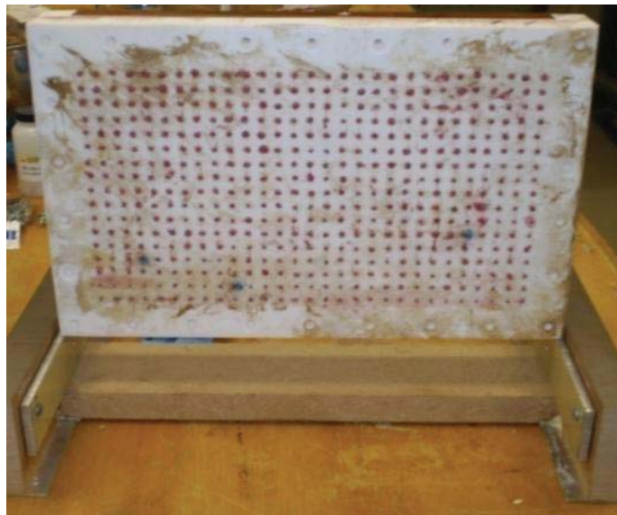
Fig. 36-Back view of the physical model to show the distribution of the copper pins, which are used to transmit the temperature from inside of the cell to outside.
