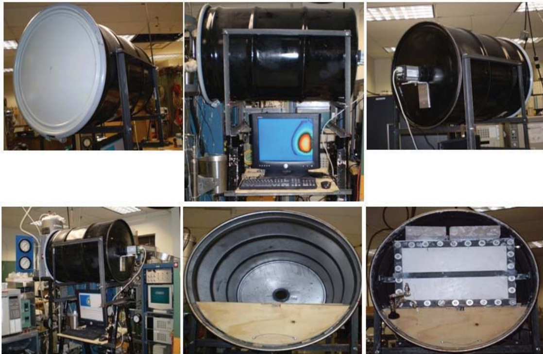
Fig. 33-Photo showing the laboratory system: the drum jacket containing SAGD cell is used to isolate the surrounding infrared noise; the concrete on the top and at the bottom of the cell is used to simulate the heat loss through over burden and under burden; the data logger under the jacket is used to record the temperature distribution from thermal camera; and the other data logger on the control panel is used to monitor the injection and production data.
