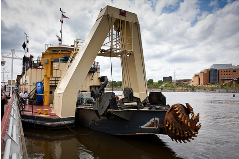
Fig. 2. Cutterhead on a pipeline dredge( U.S. Army Corps of Engineers ).
