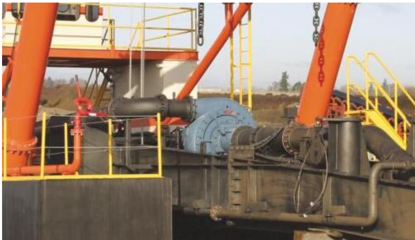
Fig. 3. Pipeline dredge centrifugal pump( Ellicott Dredges, LLC ).
