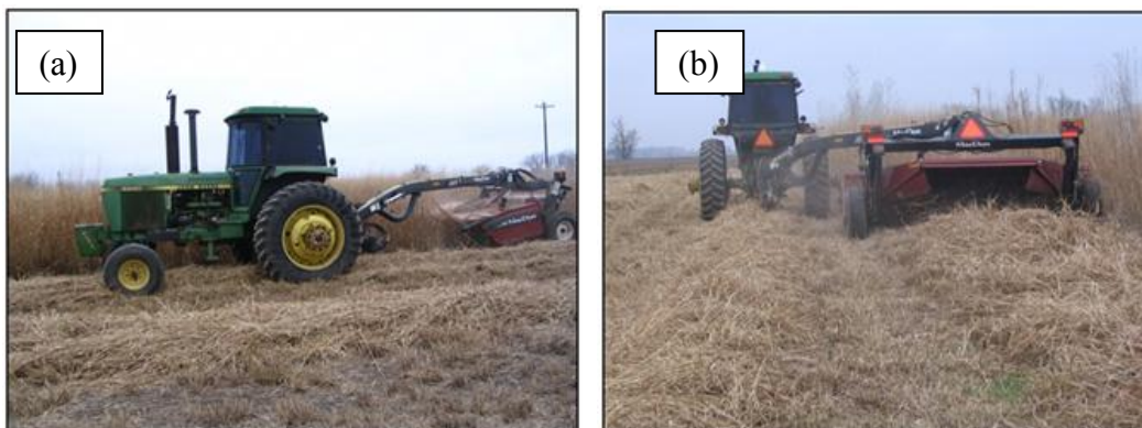
Figure 2. (a) MacDon 13' PT mower-conditioner with rotary disc header and (b) MacDon mower conditioner laying down windrows in the switchgrass field
