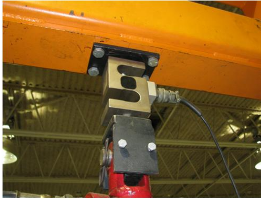
Figure 5: Hottinger Baldwin Measurement load cell
