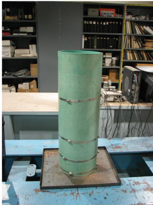
Figure 6: PVC cylinder along quick release hose clamps mounted on a metal plate
