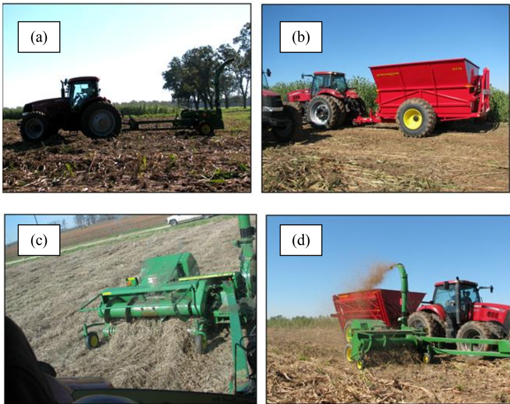
Figure 3: (a) John Deere 3955 towed forage harvester (b) Sunflower 8210 dump wagon (c) Towed harvester picking up a windrow and (d) Dump wagon collecting chopped material from the towed forage harvester
