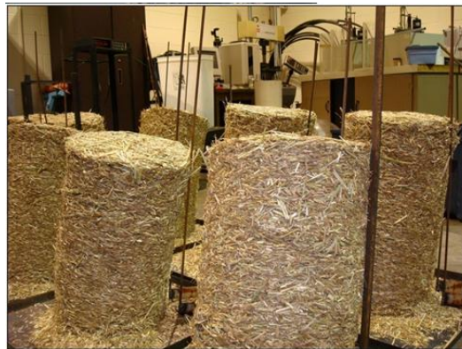
Figure 7: Switchgrass modules set aside after the compression tests
