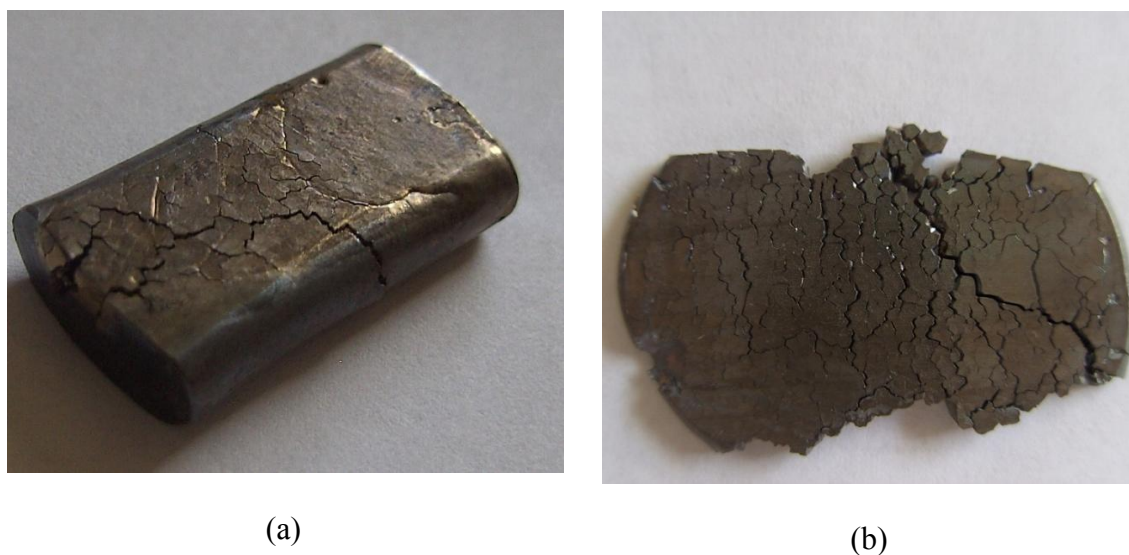
Figure 3.14 Pictures of the heavily cracked samples after hot rolling process. (a) \text{Co}_{46}\text{Ni}_{27}\text{Ga}_{27} sample heat treated at 1200^{\circ}\text{C} for 4 hrs WQ + 1000^{\circ}\text{C} for 24 hrs WQ, (b) \text{Co}_{44}\text{Ni}_{26}\text{Ga}_{30} sample heat treated at 1200^{\circ}\text{C} for 4 hrs WQ + 900^{\circ}\text{C} for 24 hrs AC. Pictures show clearly how samples cracked along grain boundaries.
