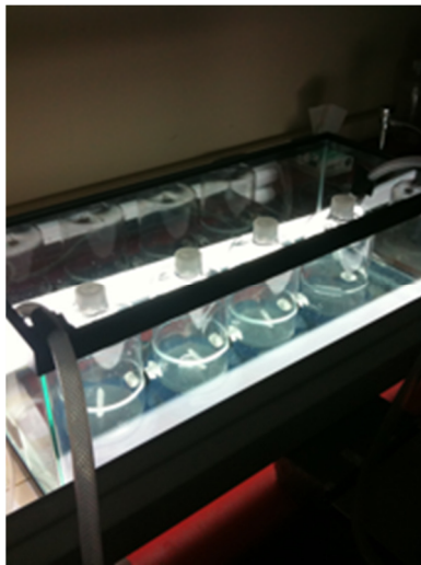
Fig. 3. Chemostat simplified diagram and setup photograph. Photograph depicts four chemostat culture vessels inside the aquarium water bath with light banks on either side. Vessels were sealed initially and before nutrient and air lines were connected.
