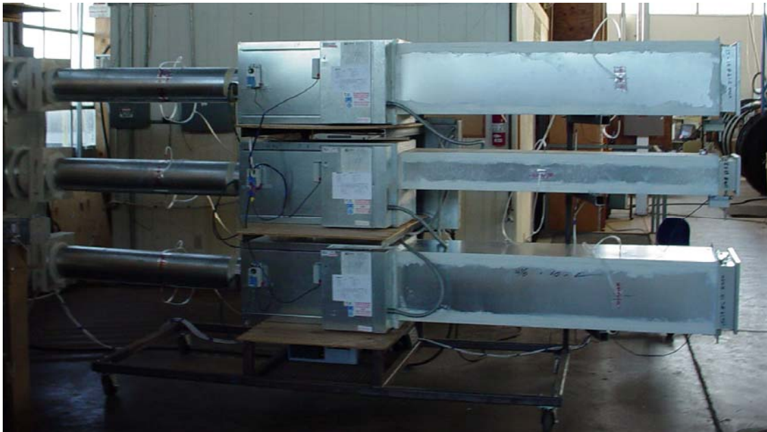
Figure V-5. Photograph of the Completed Test Stand.
