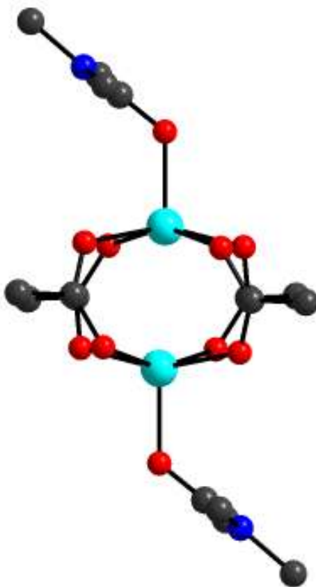
Figure 25. Zn paddlewheel of PCN-81 with solvent molecules coordinated in the axial positions.
