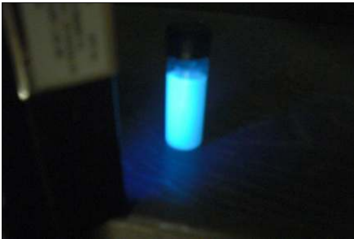
Figure 31. Luminescence of H 2 BADBA when exposed to UV lamp; pure compound dissolved in dichloromethane.
