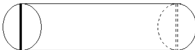
Fig. 4.58 – Sandstone Core with a Single Fracture in the Center
