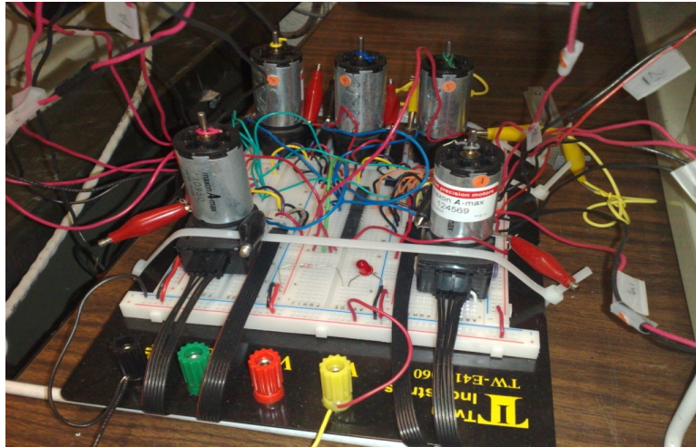
Figure 10. DC motor speed-control system
