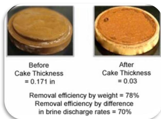
Fig. 6 —Mud cakes before/after the reaction of 10 wt% HCl with Mn_3O_4 -based filter cake, P = 250 psi, T = 250°F, and soaking time = 28 hours
