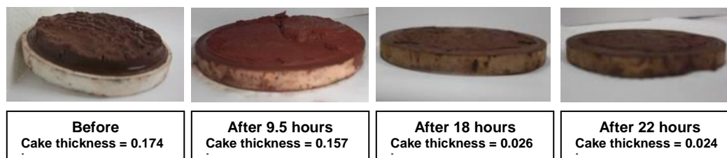
Fig. 36— Mn_3O_4 -based filter cakes before/after the reaction of (1 wt% HCl + 4 wt% lactic acid) at 250°F and 250 psi
