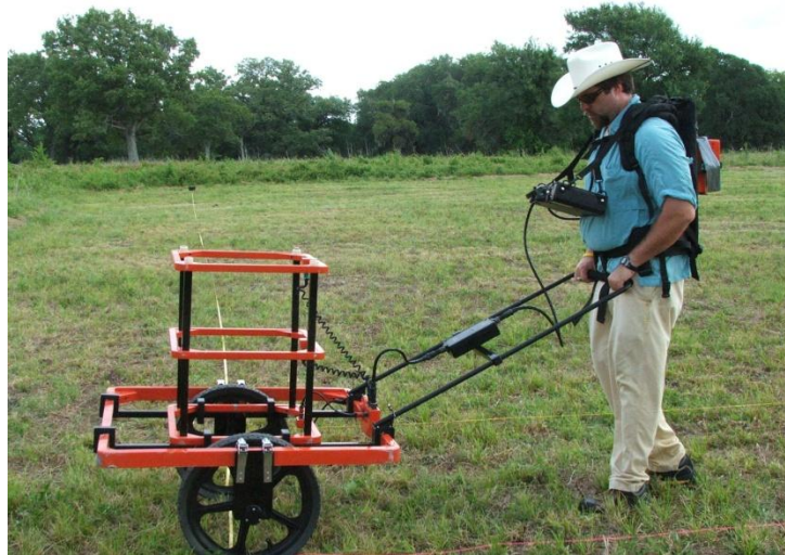
Figure 4. EM-63 being used at San Jacinto Battleground.
