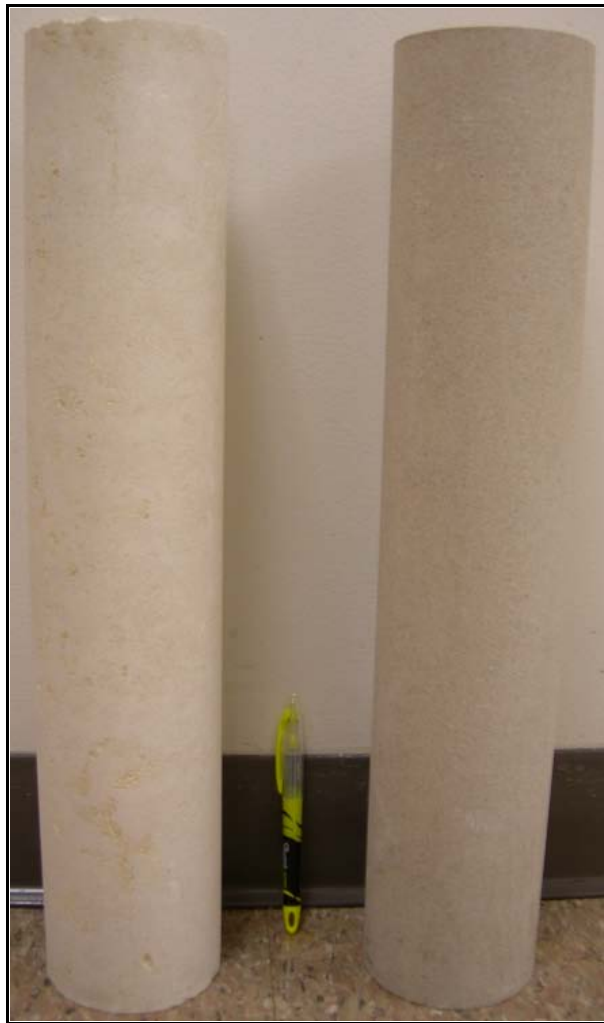
Fig. 9—Carbonate core samples (4 inches in diameter and 20 inches long).
