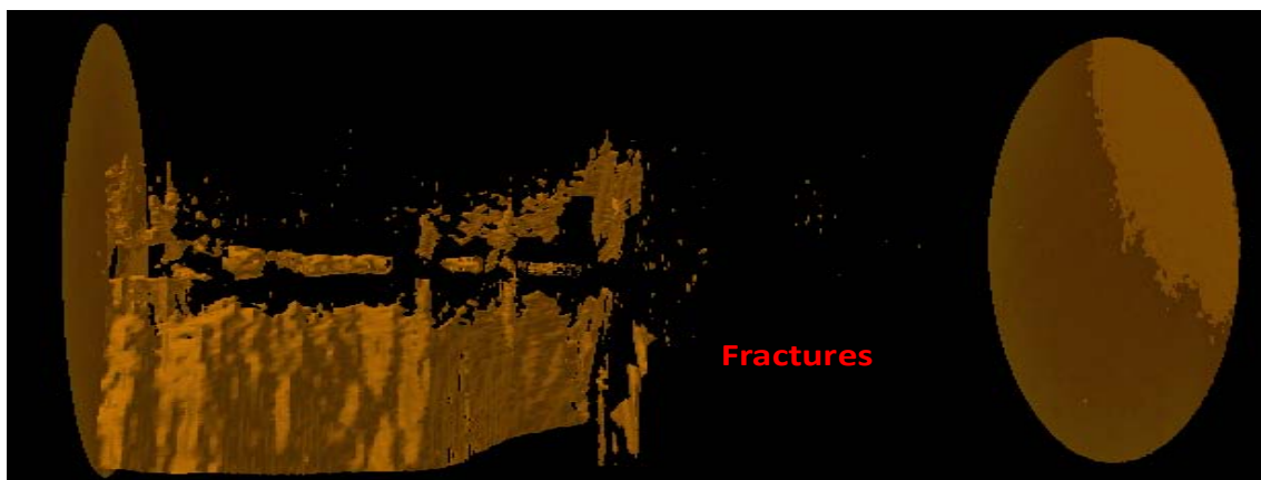
Fig. 24—3D Image of a perforated Indiana limestone core sample.
