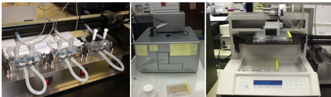
Fig. 1. Diffusion apparatus. This test bed includes three diffusion cells, a 96-well plate reader, and an automatic sampler.
