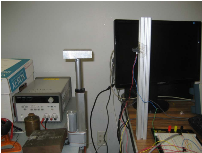
Fig. 12. The test bed of the linear actuator calibration.
